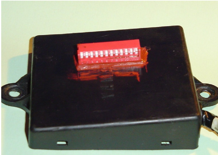
PV-Box 1WW converted to DIP-switch.
