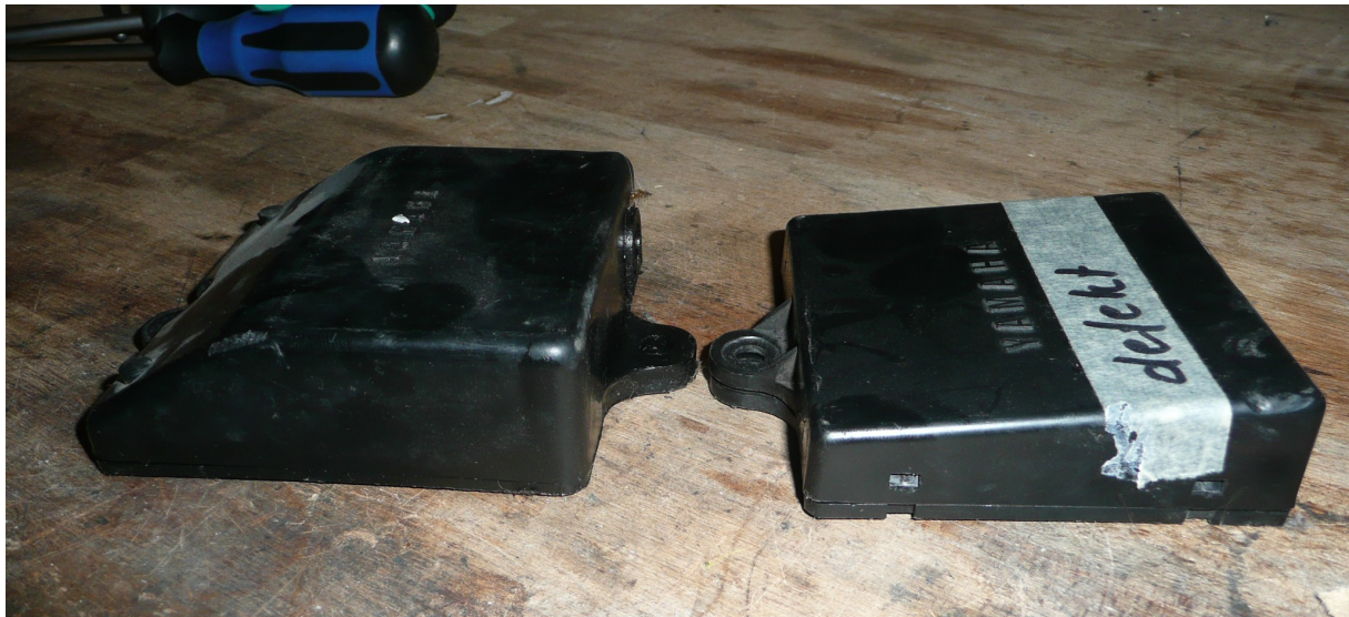
Yamaha PV boxes: left: 31K, right: later RD's, RD500, TZR250
