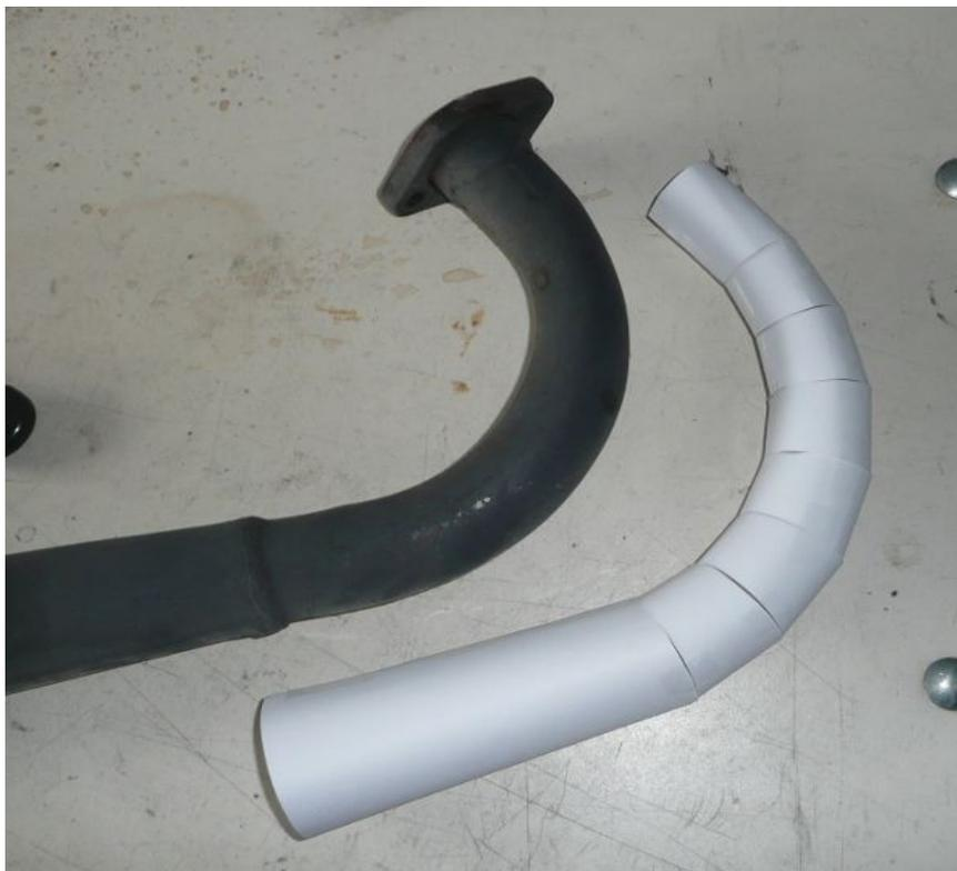
Figure 2 : Header Yamaha RD350 and paper model
