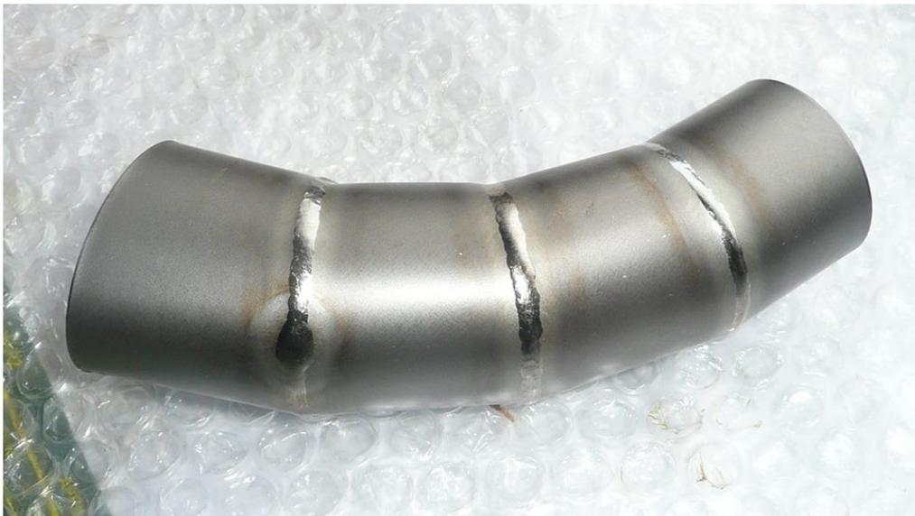
Figure 15 : Header in titanium
