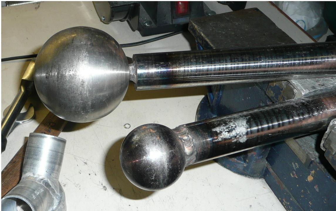
Figure 19 : Mandrel for hammering round seams
