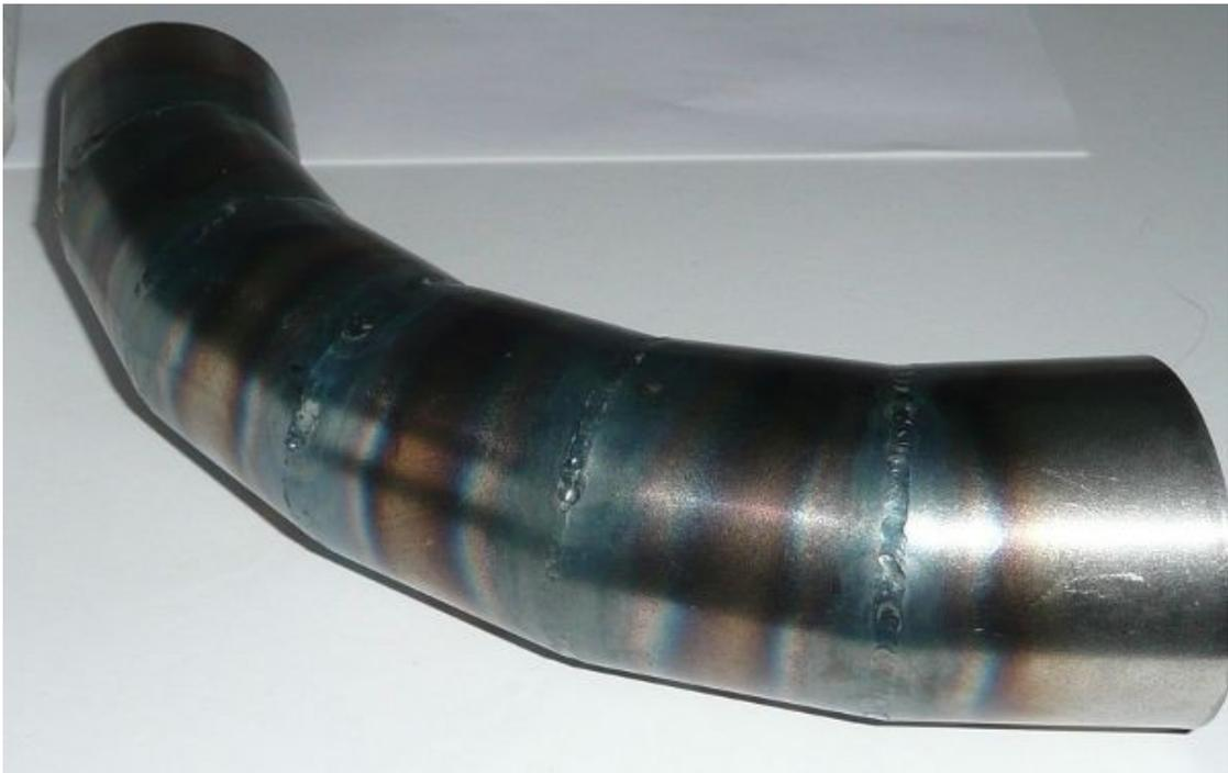
Figure 23 : Welded segments
