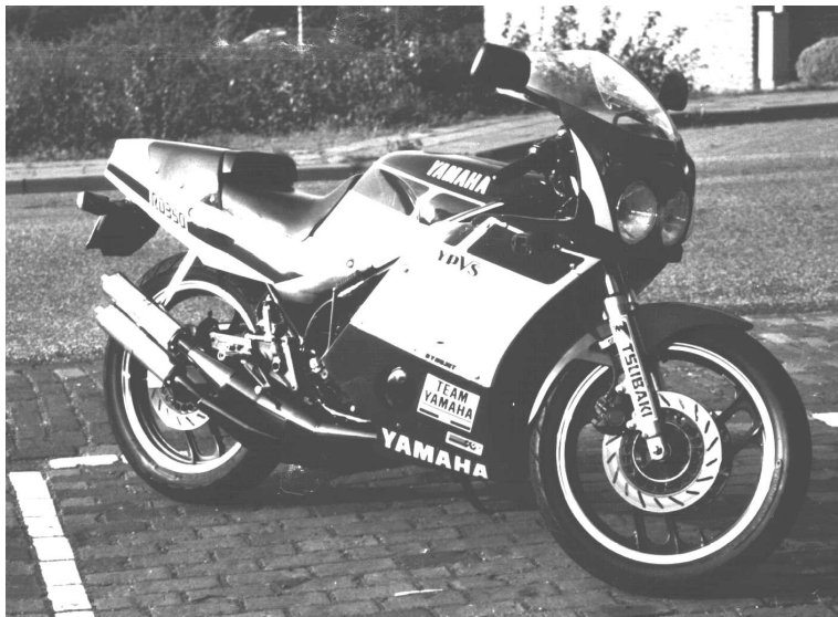
Figure 156: RZ350 English model (seen in the Netherlands), exhaust Micron Hypower
