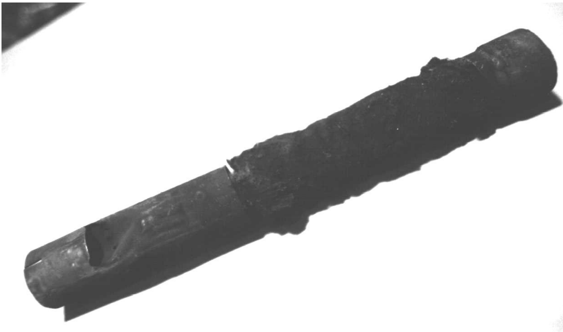
Figure 64: Silencer baffle 31K (with rockwool wrapping)
