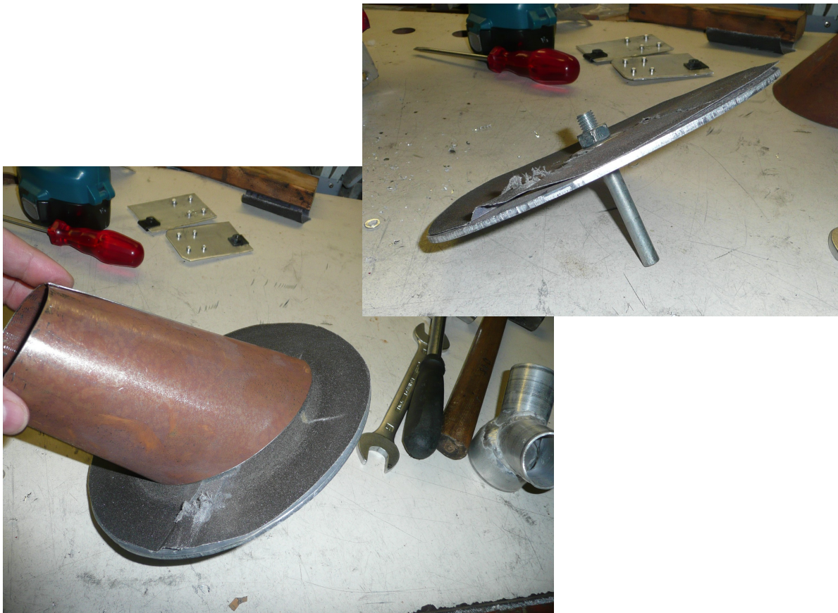
Figure 82: DIY grinding plate
