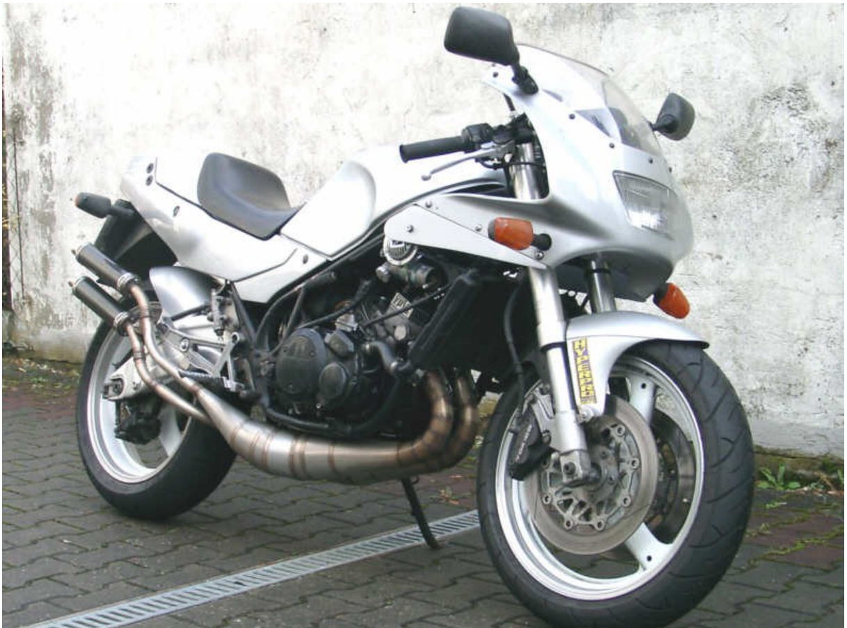
Figure 160: '86 RD350 with RGV-swingarm, fork & fairing and Soni-X GP-pipes
