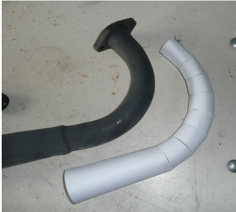
Figure 68: Header Yamaha RD350 and paper model
