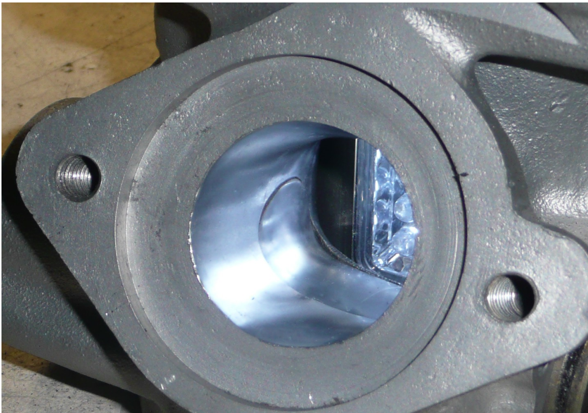
Figure 55: Exhaust port machined and polished
