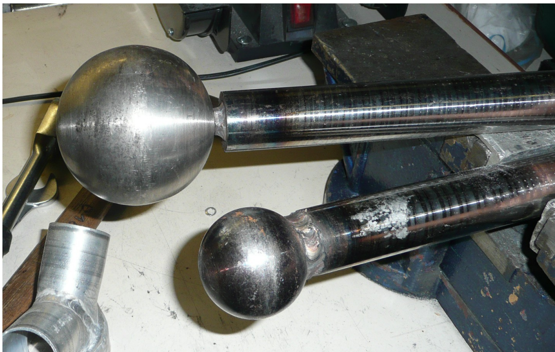
Figure 85: Mandrel for hammering round seams
