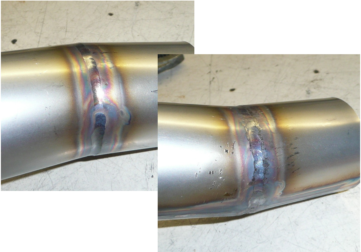
Figure 86: Finished weld before and after hammering
