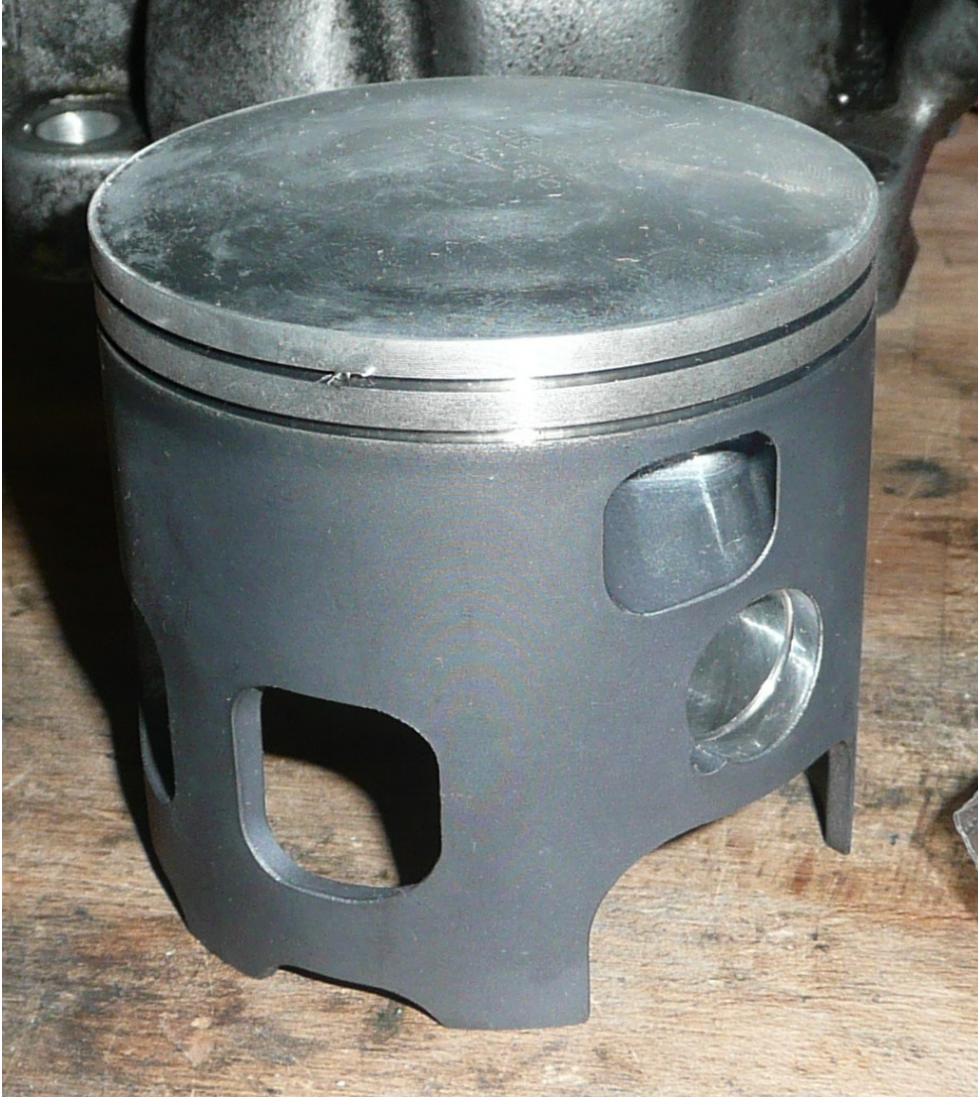
Figure 41: Woessner forged piston
