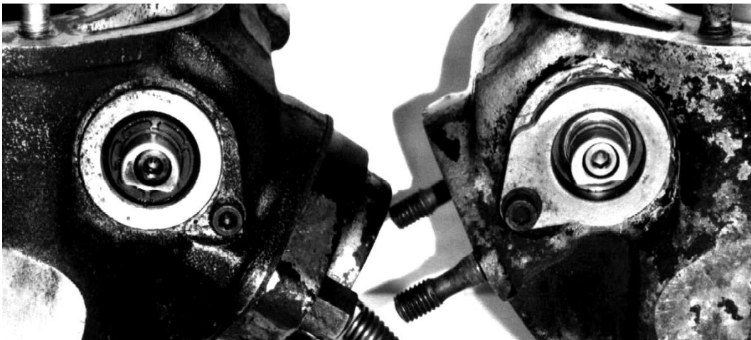
Figure 56: Inner power valve bearing bushings (Left: stock; Right: Emil Schwarz)
