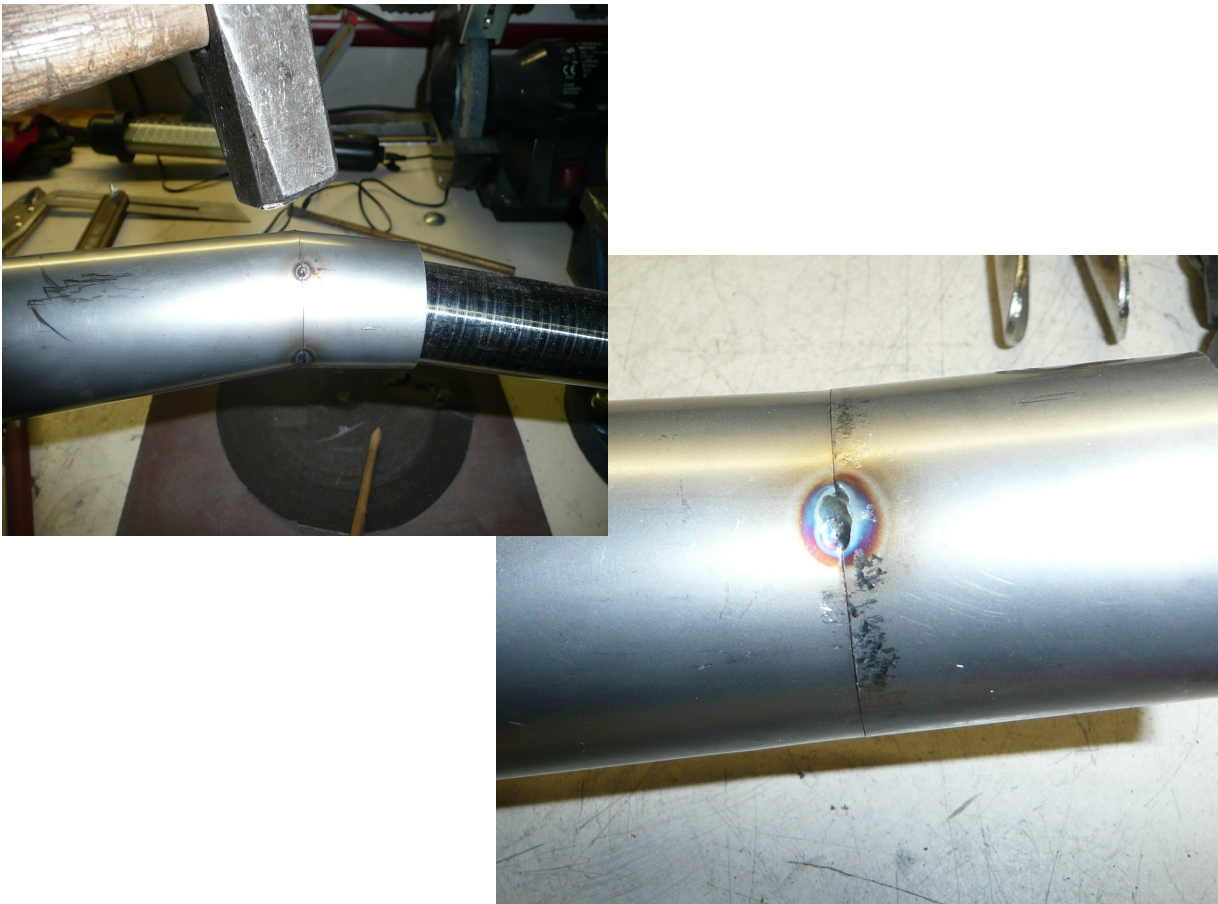
Figure 84: Hammer after tack-weld and desired perfect (=gap-less) seam.
