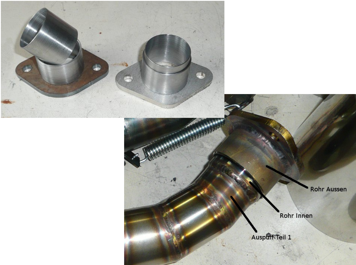
Figure 88: Cylinder flanges (DIY)
