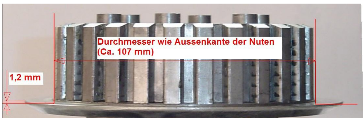
Figure 104: Modification for the hub
