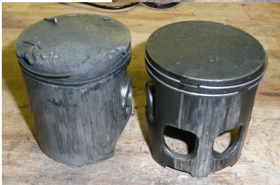
Figure 45: Some of my scrapped pistons (torn connecting rod, seizures, melted with free rings, ...)
