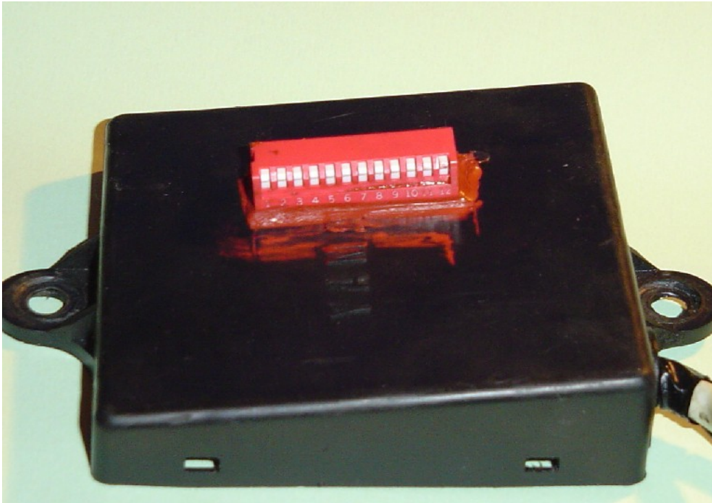
Figure 126: PV-Box 1WW converted to DIP switches
