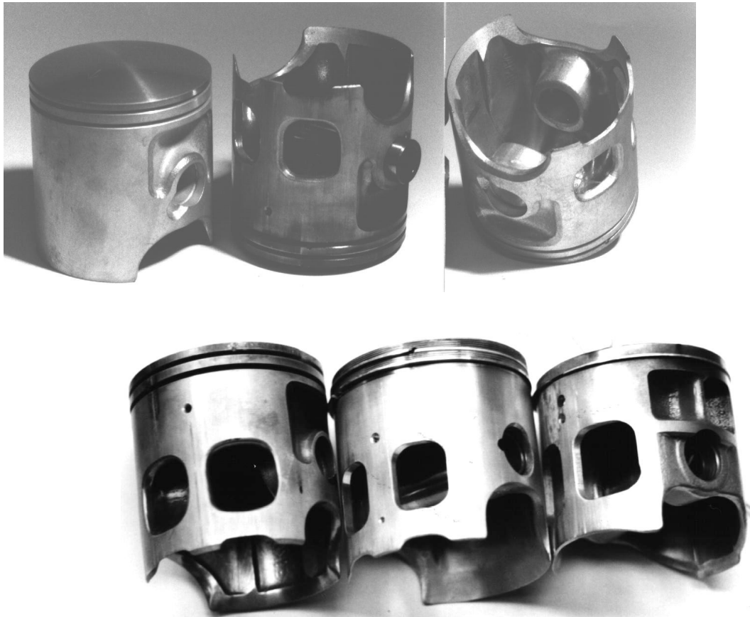
Figure 42: Modified pistons (upper row: Prox, lower row left to right: Prox, Wiseco, TZ350)
