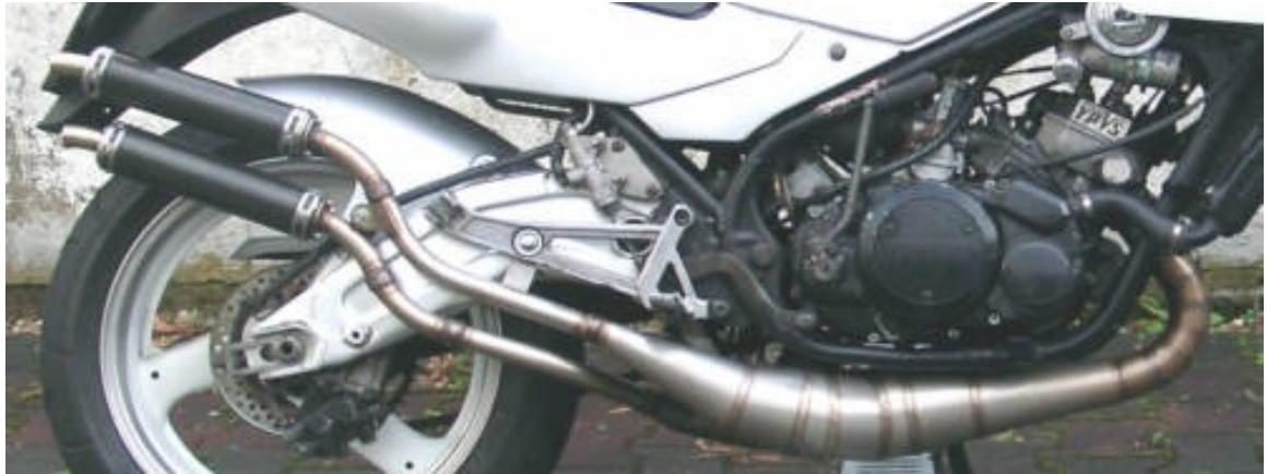
Figure 62: JL GP-Style pipes in stainless steel
