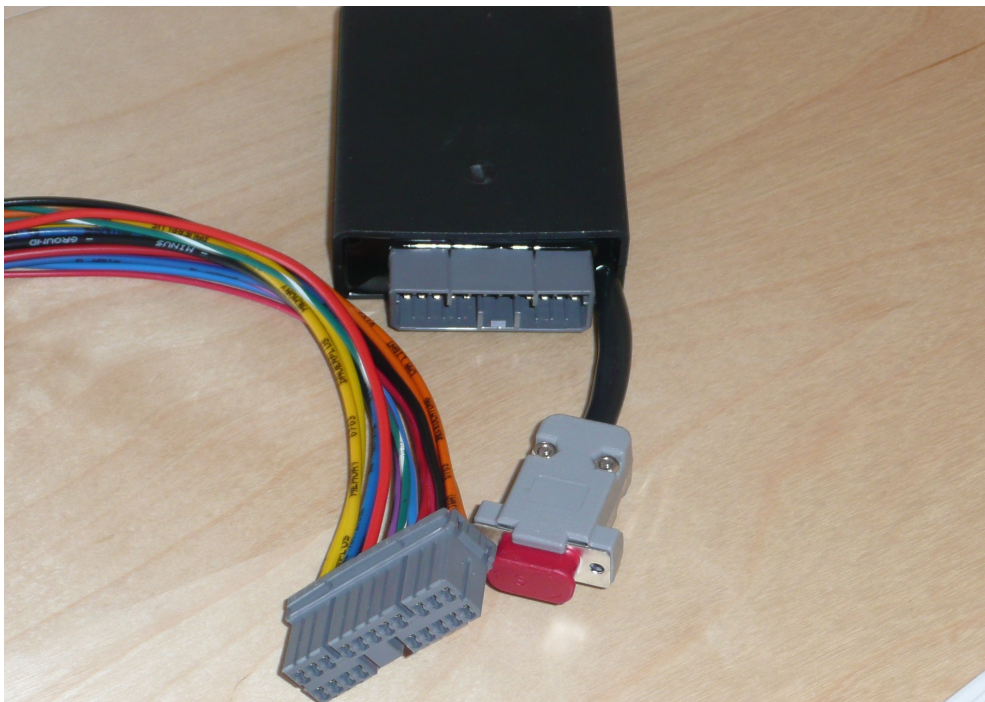
Figure 113: Ignitech DC-CDI P2 with per-fabricated harness
