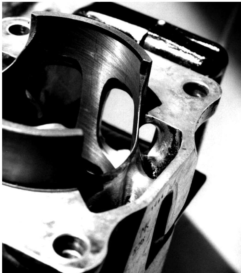
Figure 33: Boyesen port between reed region and transfer ports
