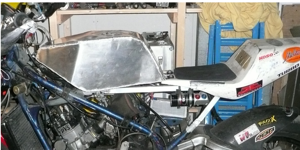
Figure 137: DIY aluminum tank and subframe
