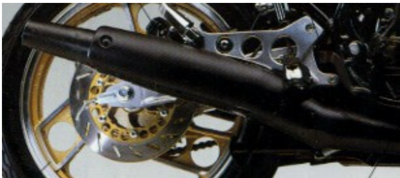
Figure 148: RZ catalyst pipes
