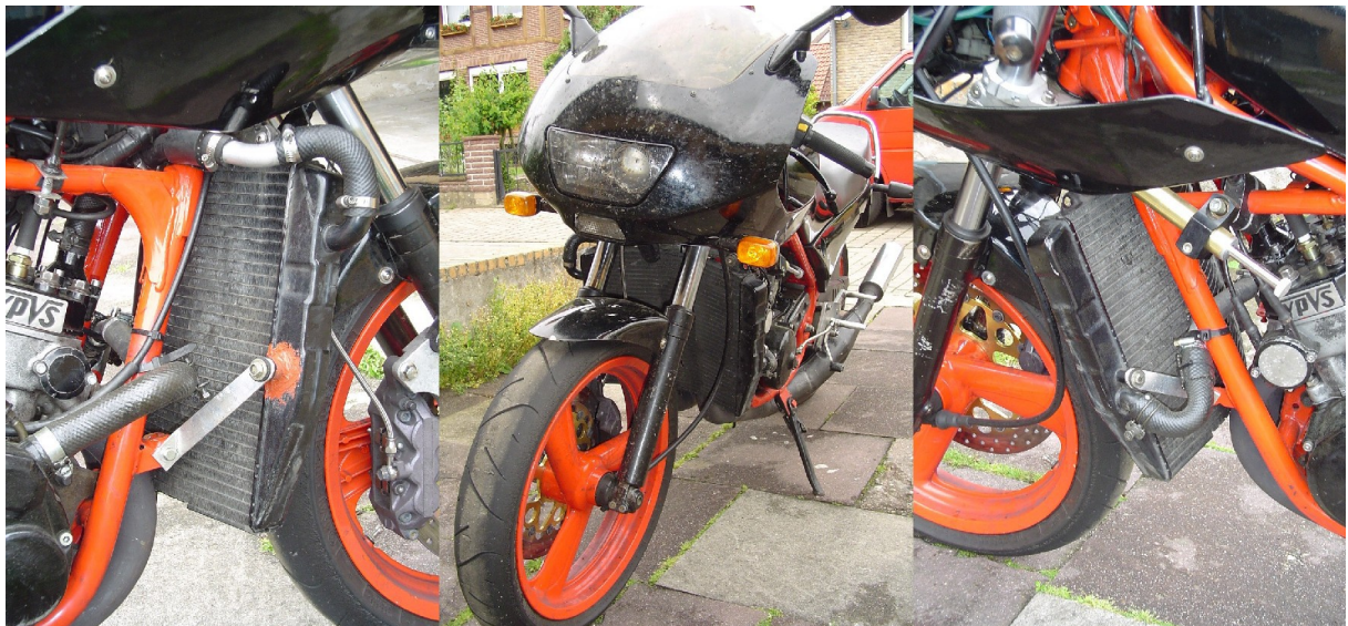
Figure 98: GSXR 1100 W radiator attached to my RD
