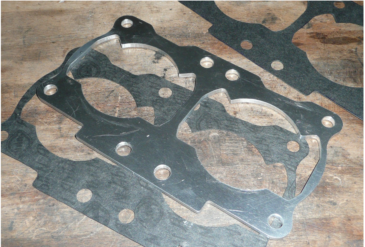
Figure 36: Cylinder base plate to compensate long rod
