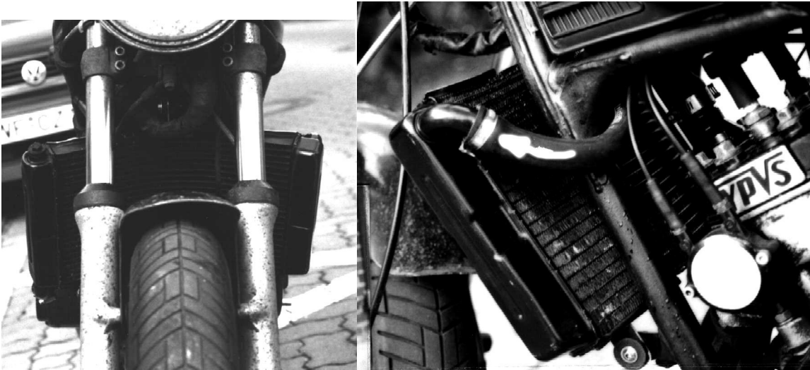
Figure 97: RGV radiator attached to my RD
