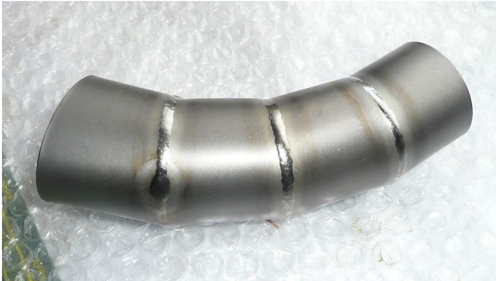
Figure 81: Header in titanium
