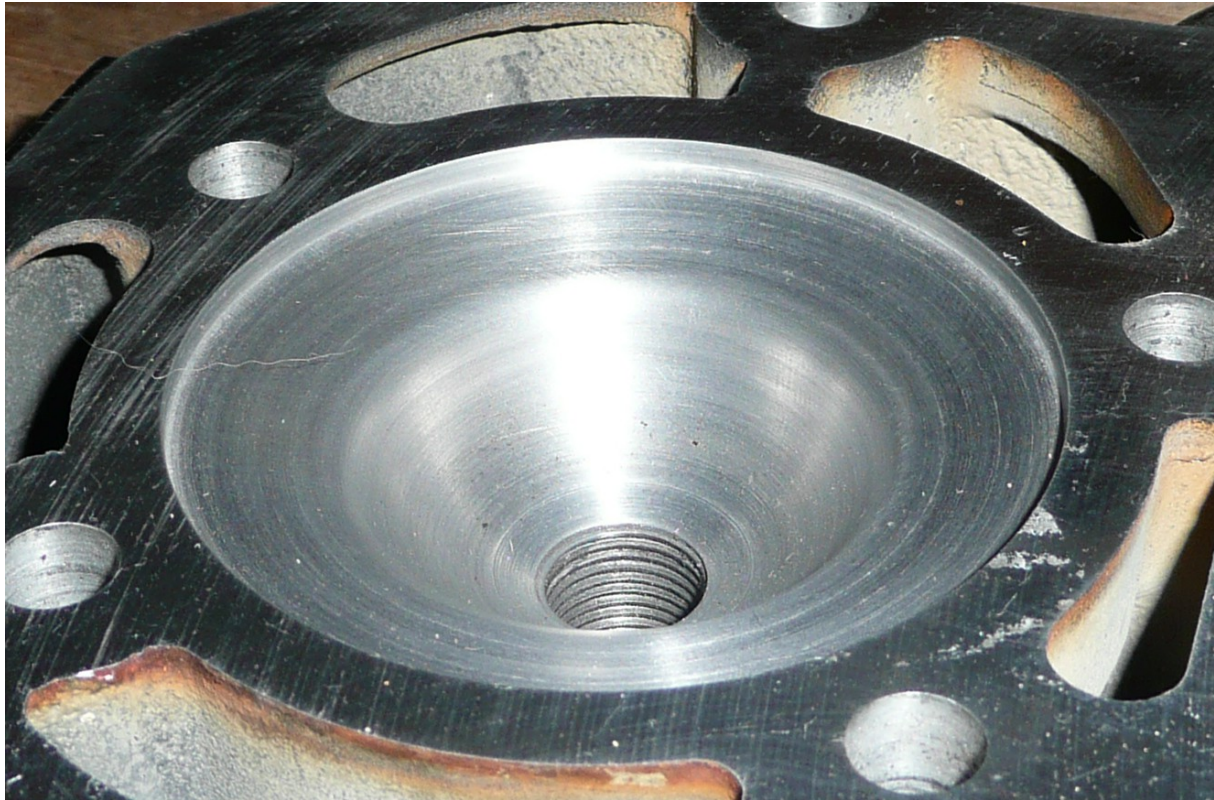
Figure 37: Head mod for a +4 crank
