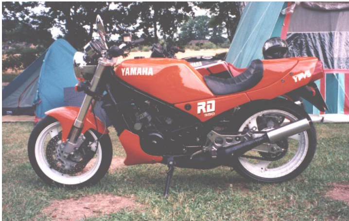
Figure 151: 31K with RGV fork, GPZ 600R swingarm
