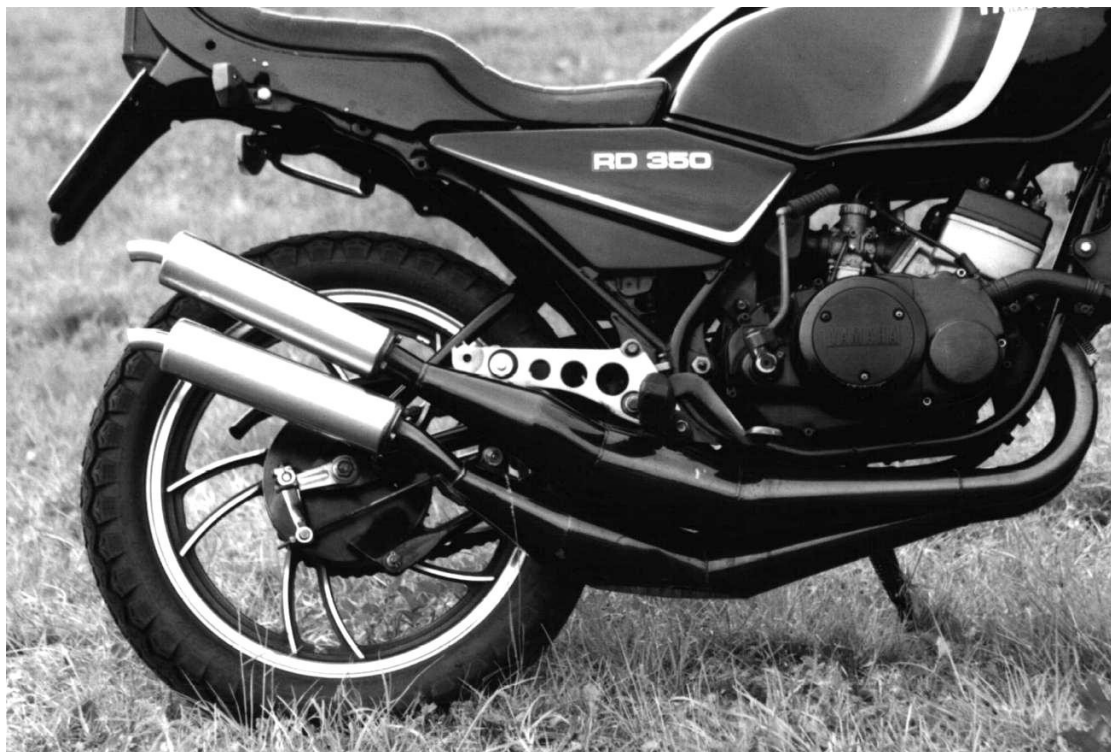
Figure 63: Micron Hypower (originally this was sold for the RD350YPVS but as you see it fits well to the RD 350 LC, too)
