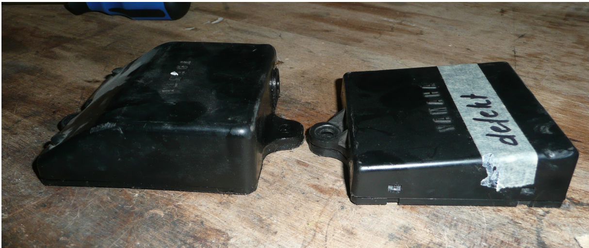
Figure 121: Yamaha PV boxes: left: 31K, right: later RD's, RD500, TZR250
