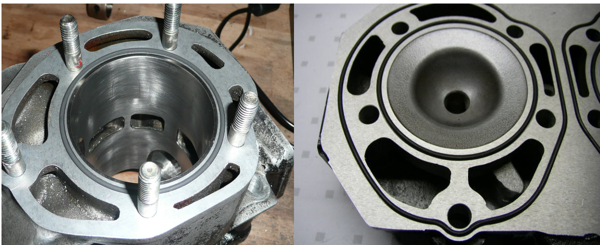
Figure 3: O-Ring conversions (Left: single ring in cylinder, Right: dual rings in head)
