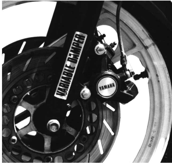
Figure 143: RD500 caliper on 1WW
