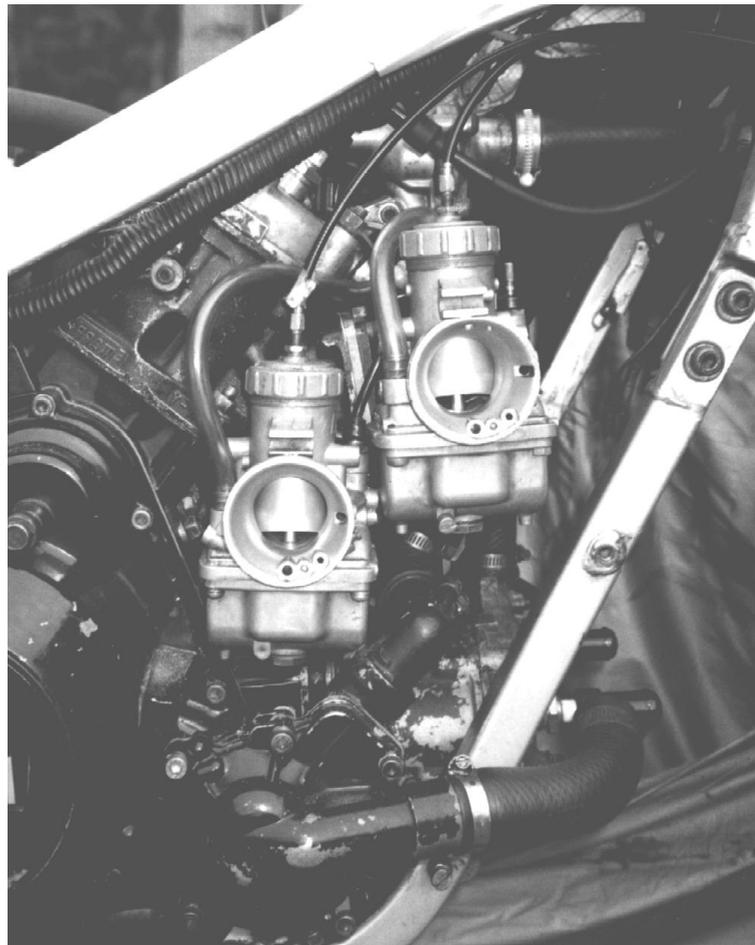
Figure 32: VM34 mounted to the engine
