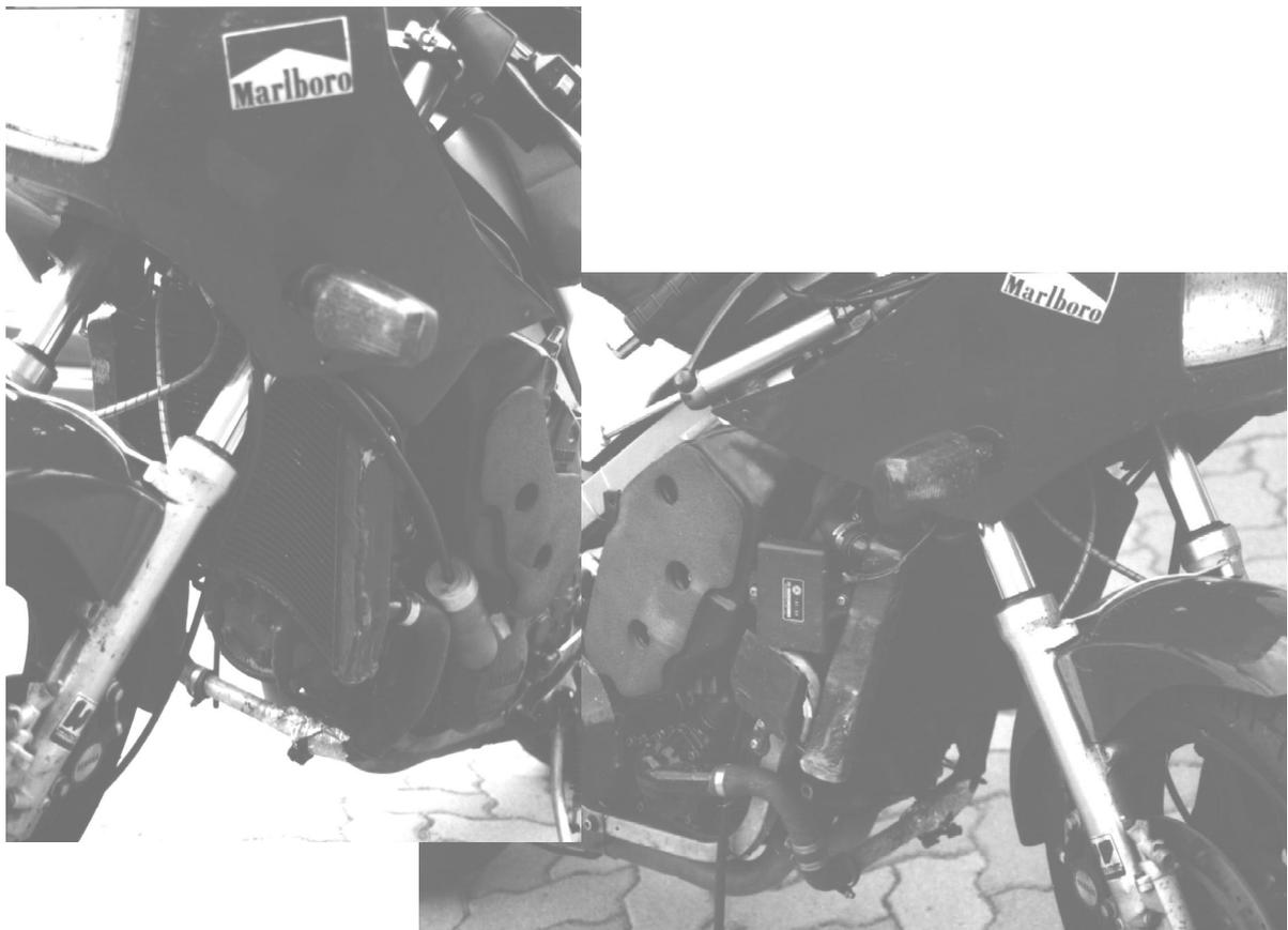
Figure 79: GXSR750W radiator fit to RD500
