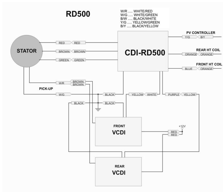
Figure 87: Wiring with two VCDI's (front/rear bank with separate advance curves)
