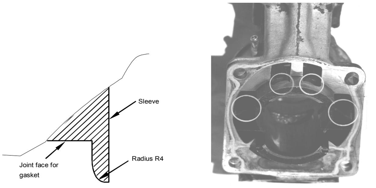
Figure 51: Upper cylinder, stock sleeve
