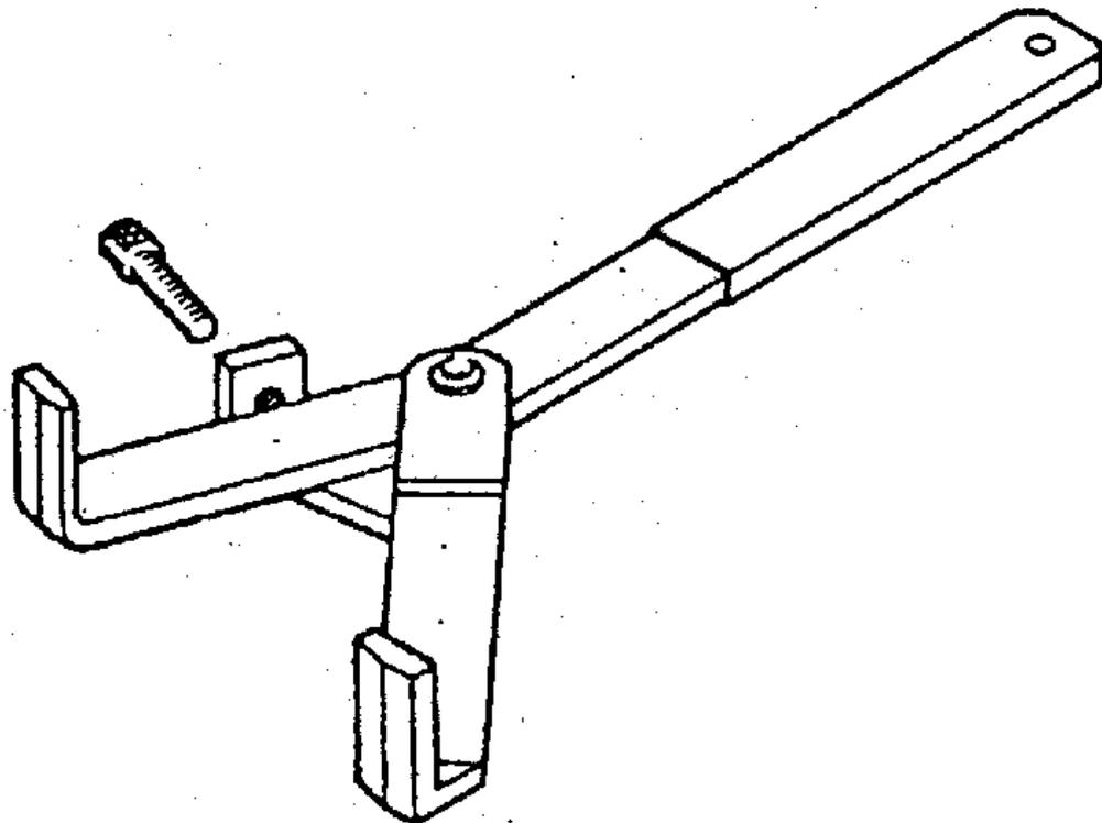
Figure 114: Clutch holding tool
