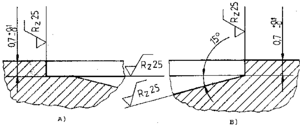
Figure 66: Reworked squish-area; A) The easy way: edge with 90° and 0.7 mm height. ; B) The better way: angle of 15° remains.
