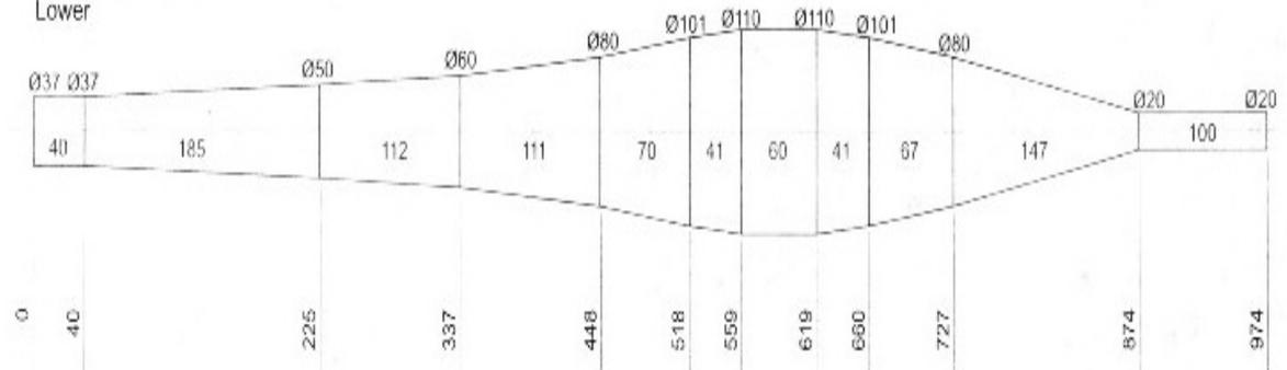
Figure 72: YAMAHA race pipe dimensions
