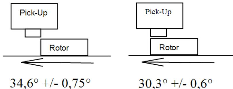
Figure 89: Reference position Pickup/Rotor (left)
