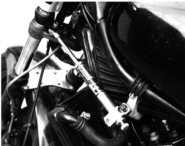
Figure 102: Steering damper (RD350)
