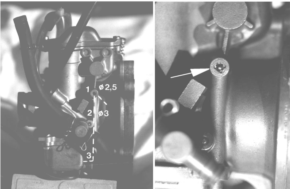
Figure 20: Left: passages in the carb, Right: closed end of passage 1
