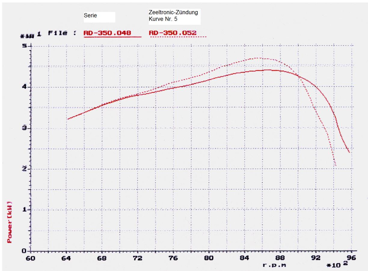
Figure 88: RZ350 Dyno curves (rear wheel power) for stock and modified advance curve.
