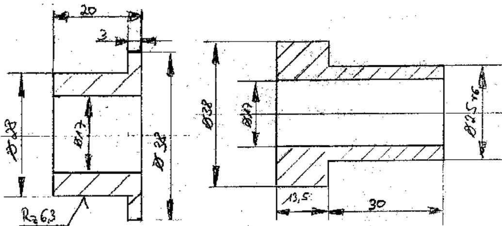
Figure 118: Right wheel spacer and brake carrier spacer
