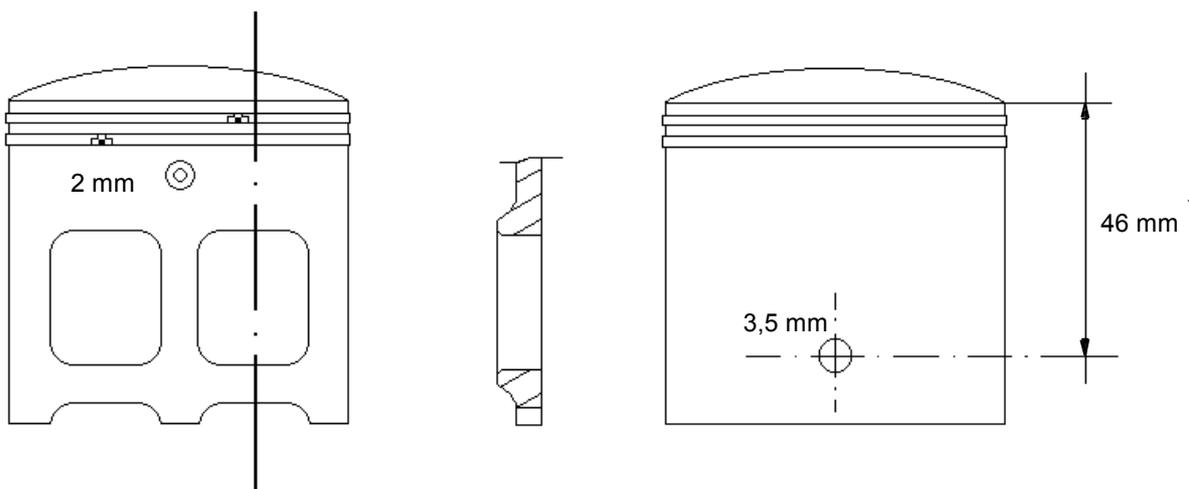
Figure 55: Piston lubrication holes
