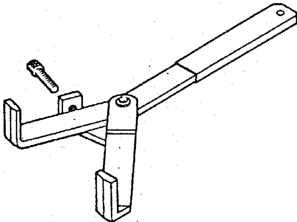
Figure 114: Clutch holding tool
