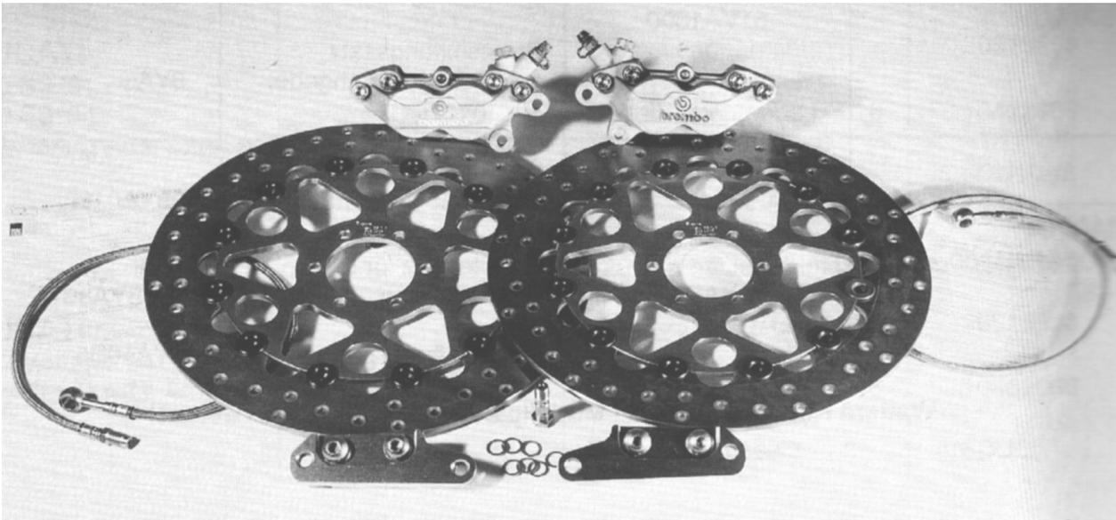
Figure 99: Brembo 4 piston caliper Kit (Courtesy of Brune catalogue)
