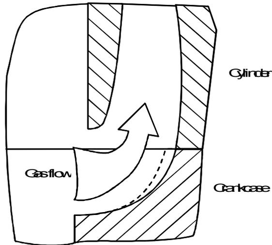
Figure 49: Section through cylinder and crankcase along the scavenging-port
