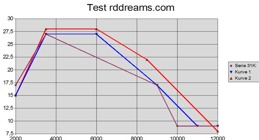
Figure 85: Advance curves used for CDI prototype (31K = Stock RZ350 curve)
