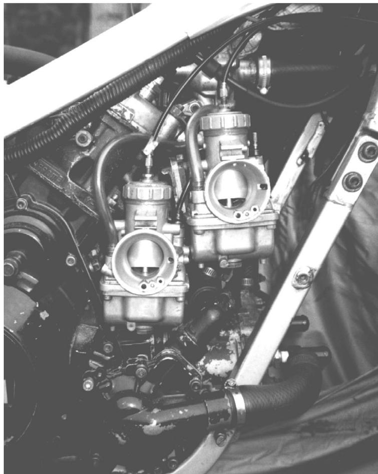
Figure 32: VM34 mounted to the engine
