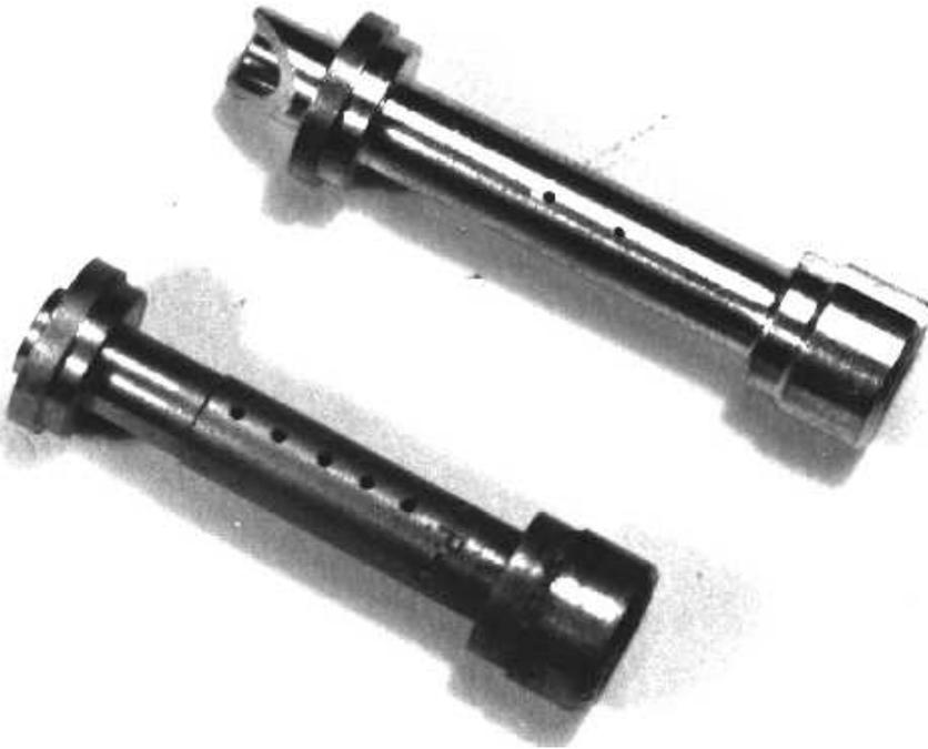
Figure 17: Nozzles, front RD350 O-0, rear: Ledar intake kit
