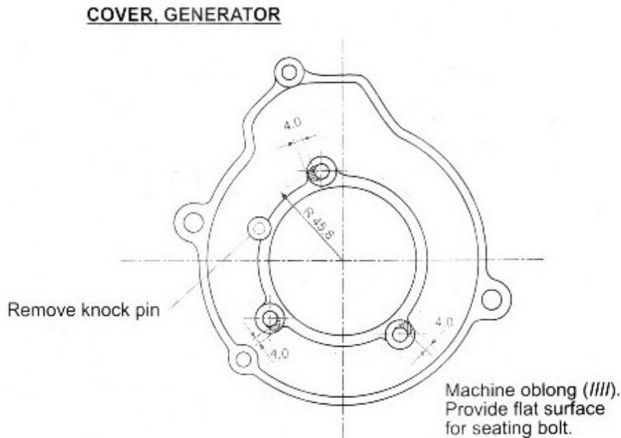
Figure 83: Advance ignition by generator cover modification (YAMAHA race specs)
