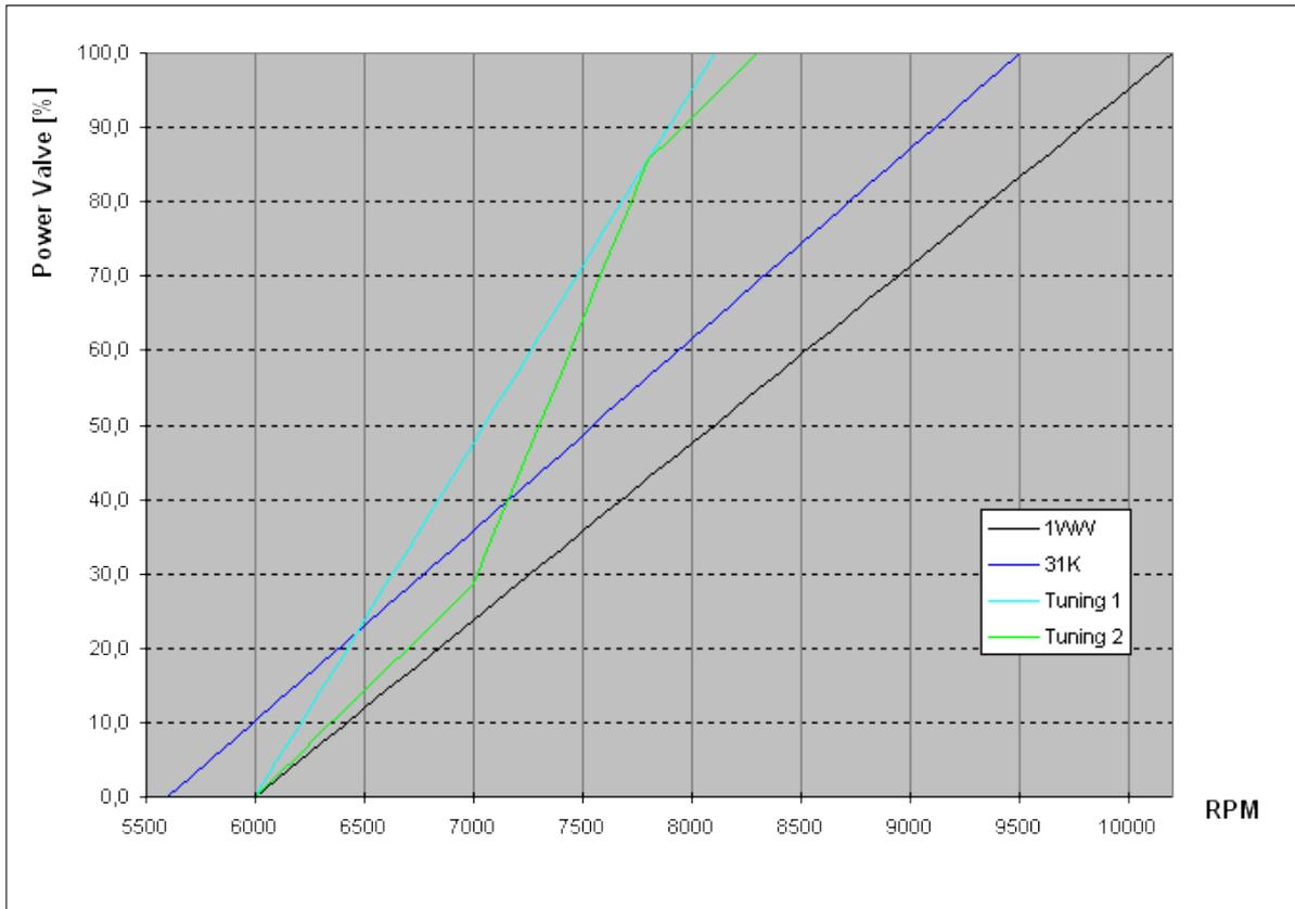
Figure 93: Opening examples for RZ350 (1VW/31K Stock, Tuning 1/2 from Hans K.)
