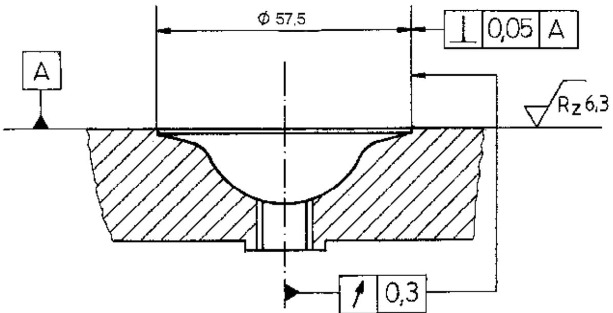
Figure 65: Cross-section of the cylinder head with rework dimensions
