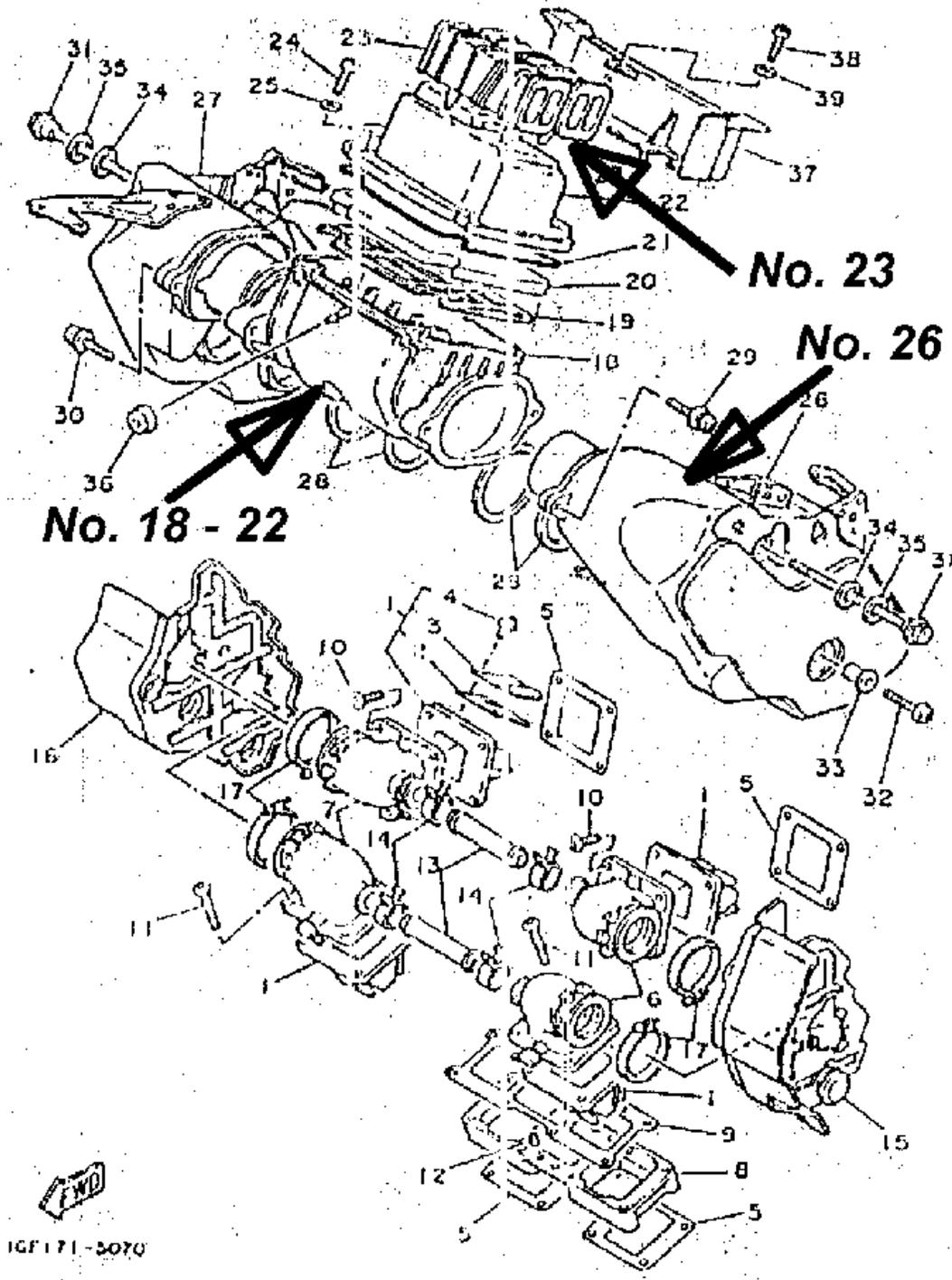
Figure 16: Stock air filter (rubber snorkels No. 23, elephant ears No. 26/27, top air filter housing No. 18 – 22)
