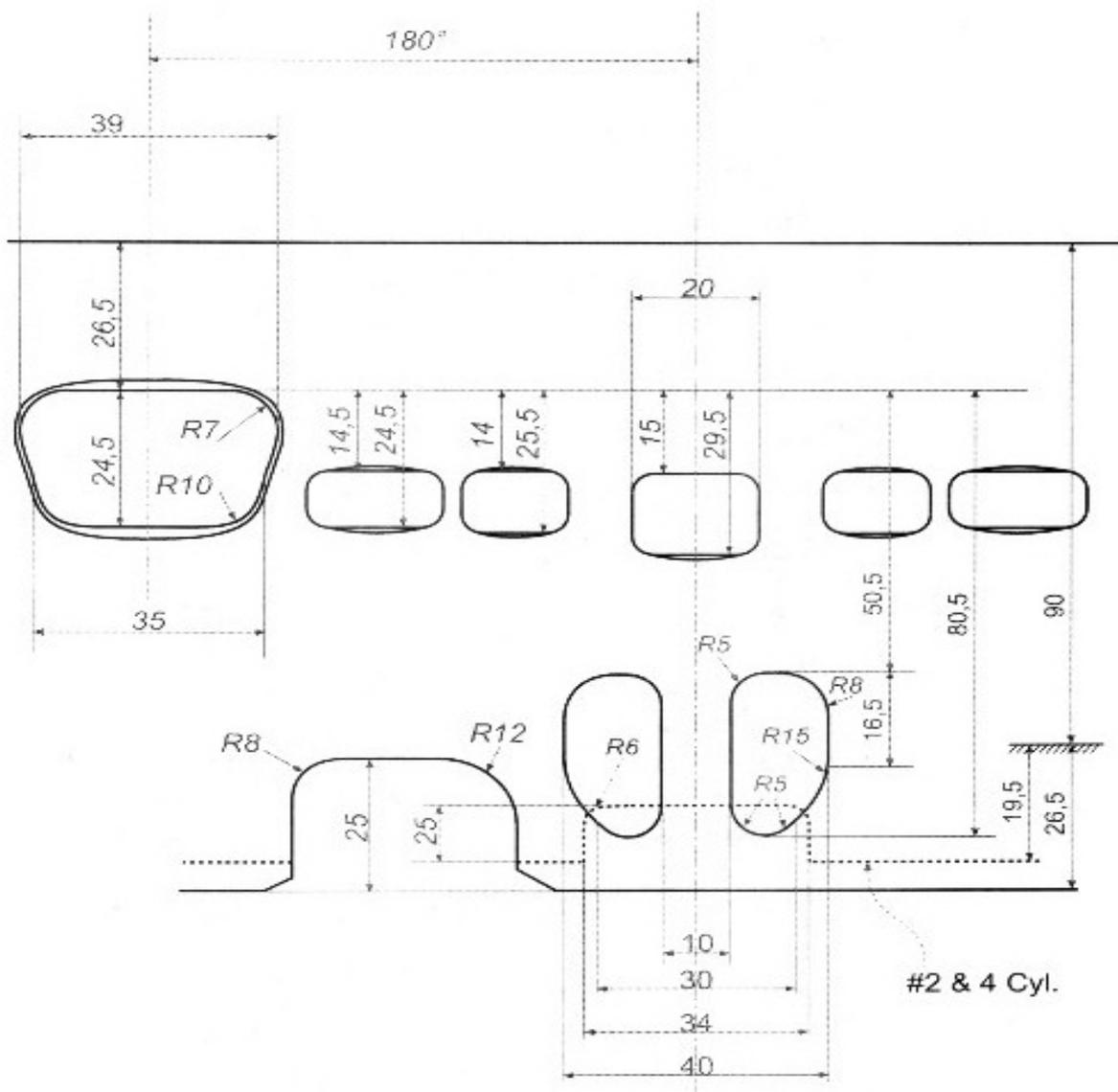
Figure 74: Stock port configuration (YAMAHA race specs)
