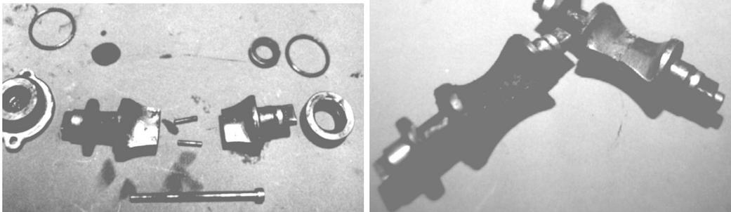
Figure 5: YPVS Valves (unmounted, with and without carbon coating)
