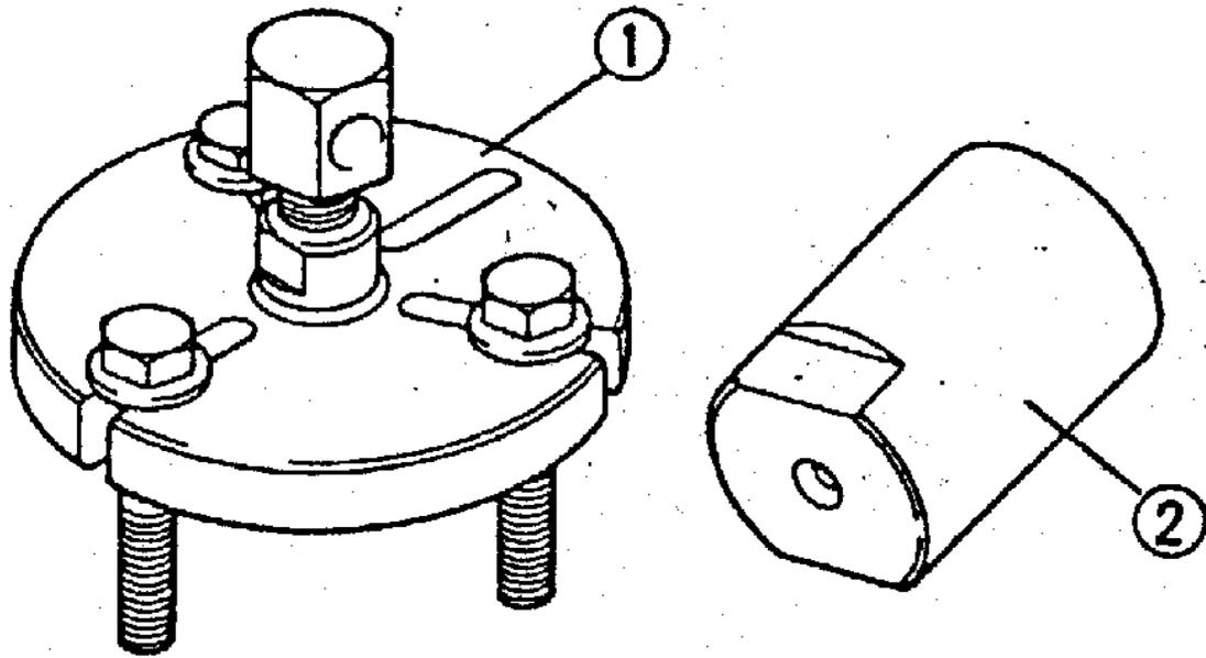
Figure 113: Flywheel puller tool
