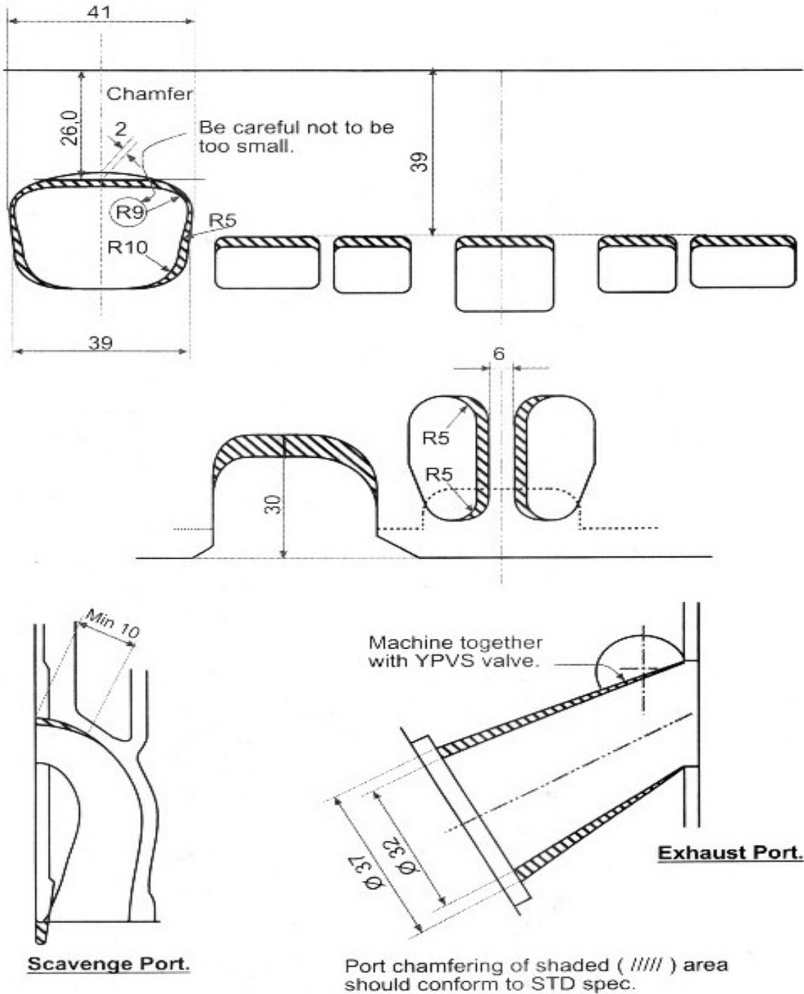
Figure 75: Modified port configuration (YAMAHA race specs)
