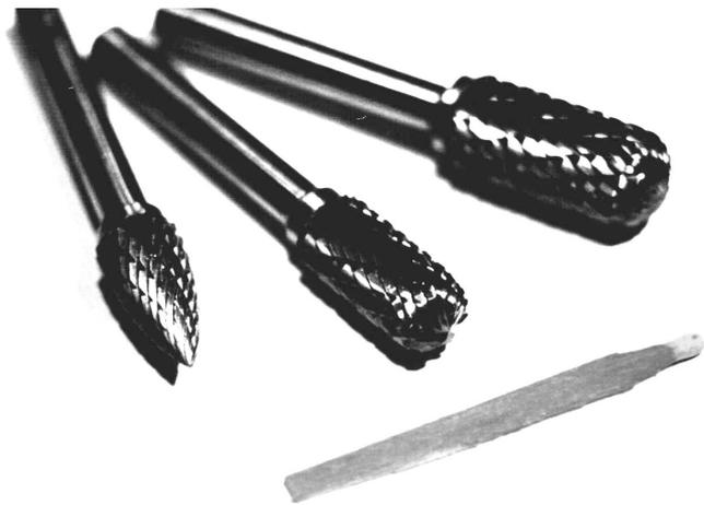
For the exact finishing and deburring of the port shapes at the sleeve you have to use the file set.
