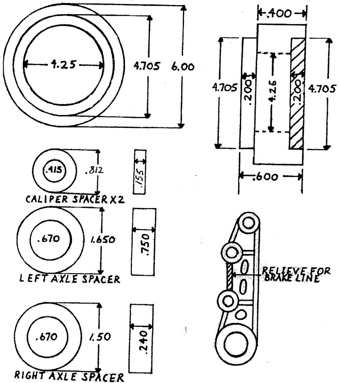
Figure 116: Usage of FZR600 rear wheel in RD500 stock swingarm (courtesy of Ron Atchinson / RD500 newsletter April 98), Dimensions given in inch
