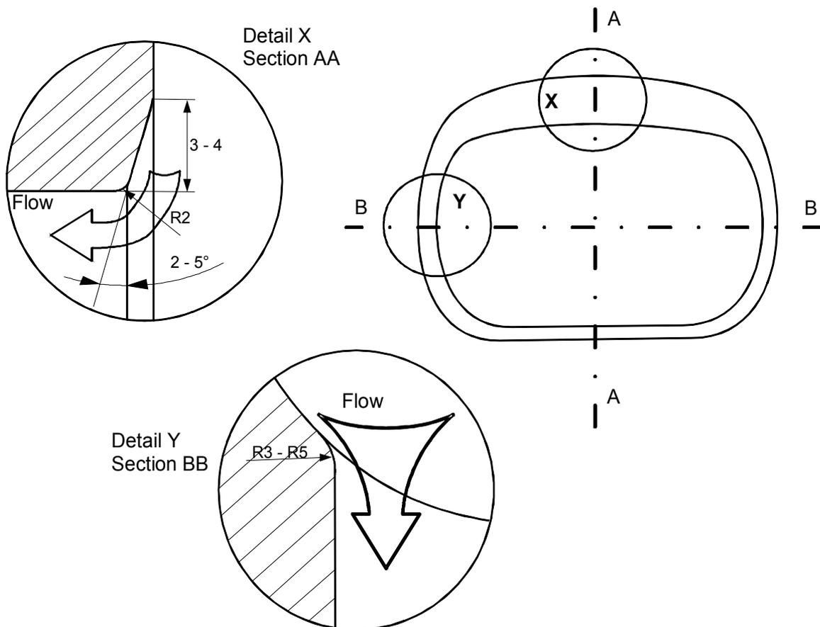
Figure 69: Details of chamfering and radii at port edges
