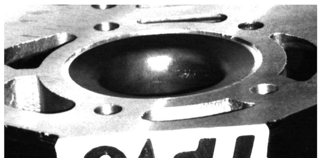
Figure 63: Milled cylinder head with reworked 0.7 mm straight (RZ350)
