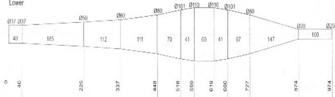
Figure 72: YAMAHA race pipe dimensions
