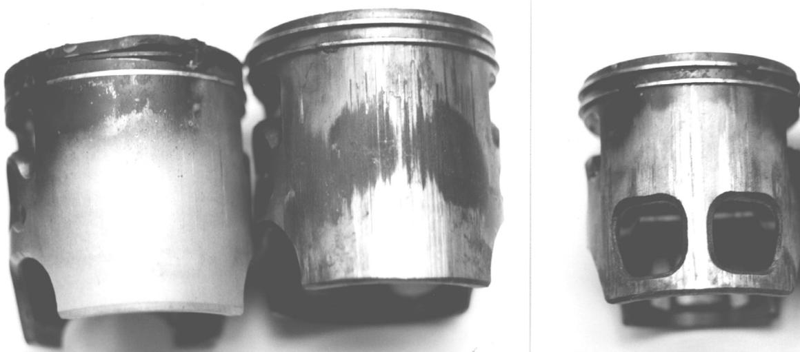
Figure 56: Damaged pistons: left: broken ring, middle/right: seized
