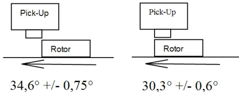
Figure 89: Reference position Pickup/Rotor (left)
