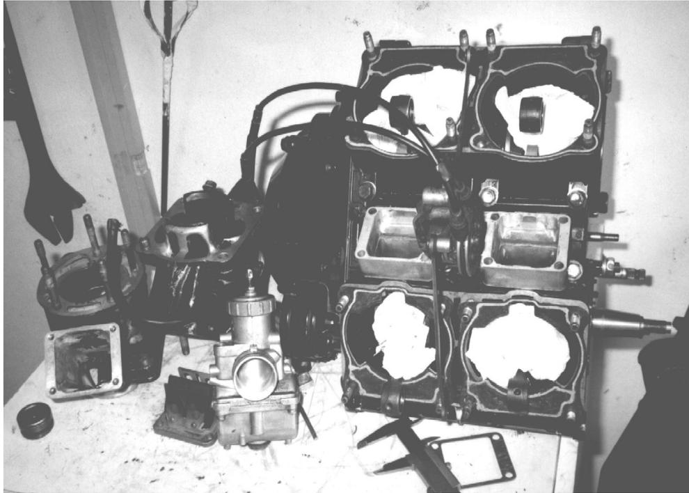
Figure 31: Engine view (sleeve mods, reed cages, reed housing lower cylinder bank)
