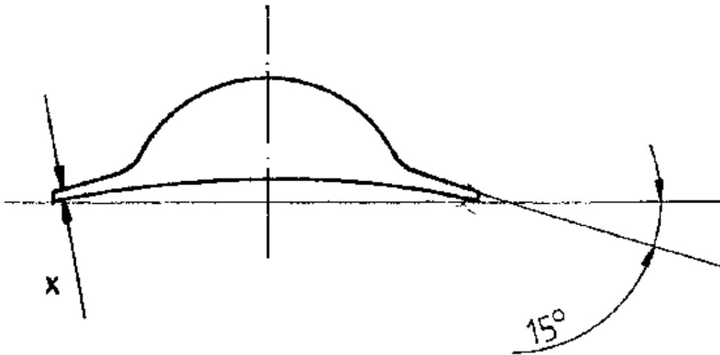
Figure 64: Cross-section of the stock combustion chamber in TDC position
