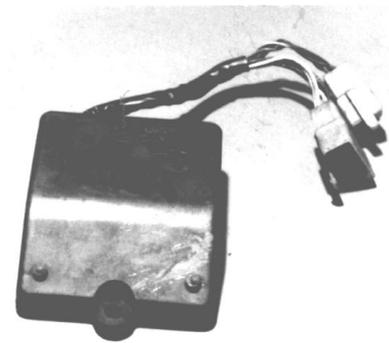
Figure 12: YPVS control unit RD350 (31K)
