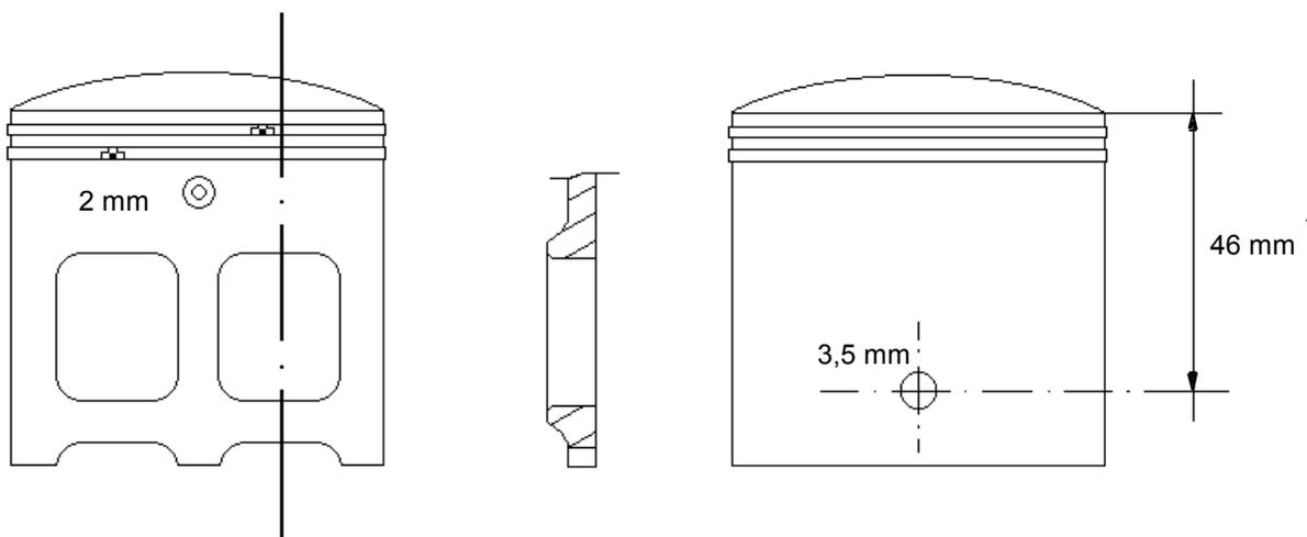
Figure 55: Piston lubrication holes
