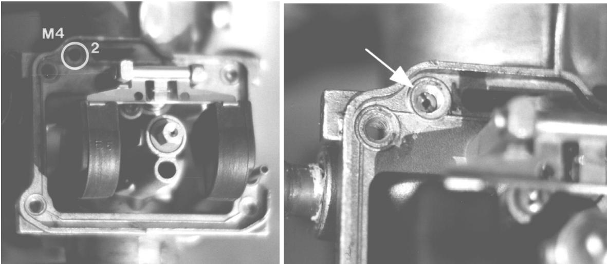
Figure 19: End of passage 2 (left: stock, right: modified)
