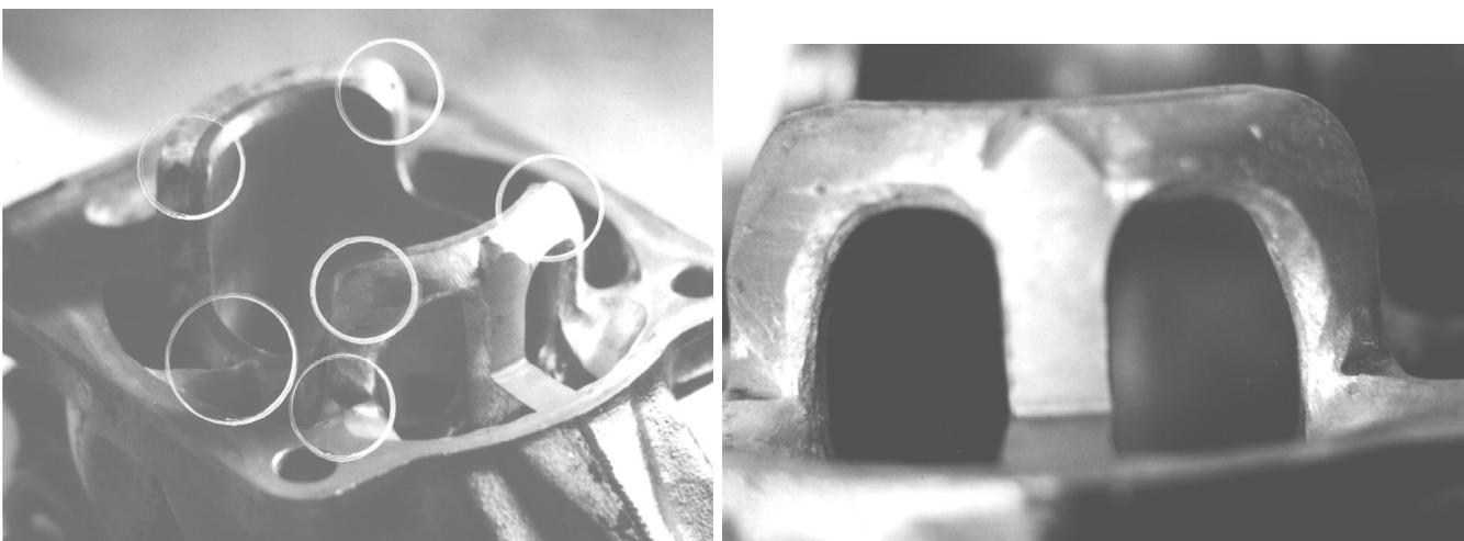
Figure 52: Upper cylinder, modified sleeve
