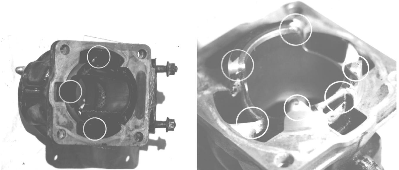
Figure 53: Lower cylinder, left: stock, right: modified
