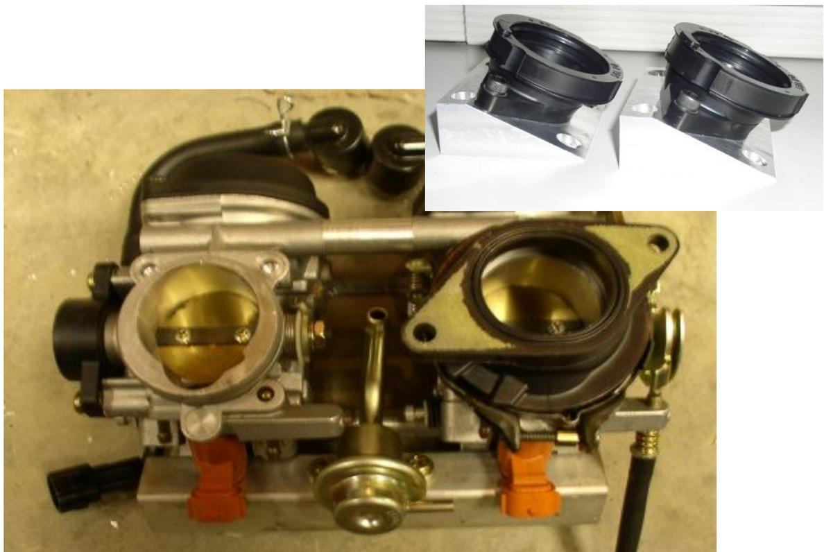
Figure 36: R6 Manifolds, throttle bodies & pressure regulator reworked to fit the RZ350.
