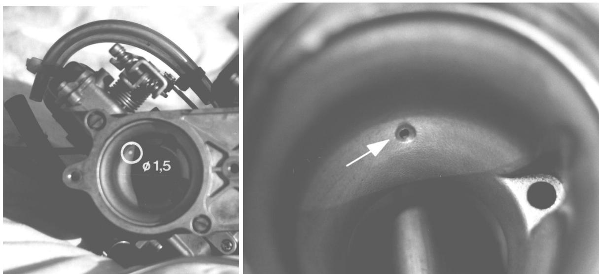
Figure 18: Power jet discharge location (left: stock, right: modified)
