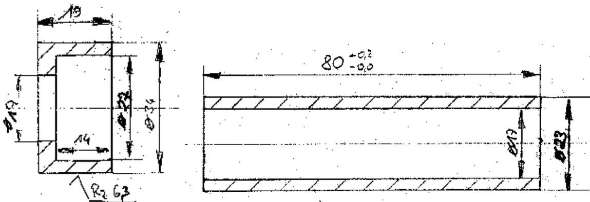
Figure 117: Left Wheel spacer and bearing spacer (between wheel bearings)
