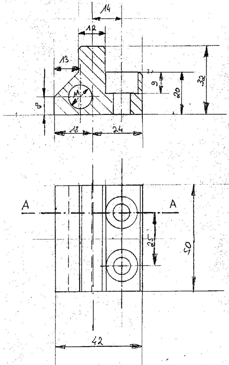
Figure 121: Brake anchor at the swingarm (mount with plate with two welded nuts)
