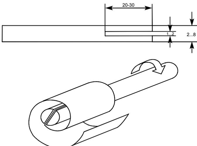
Figure 2: Polishing shaft
