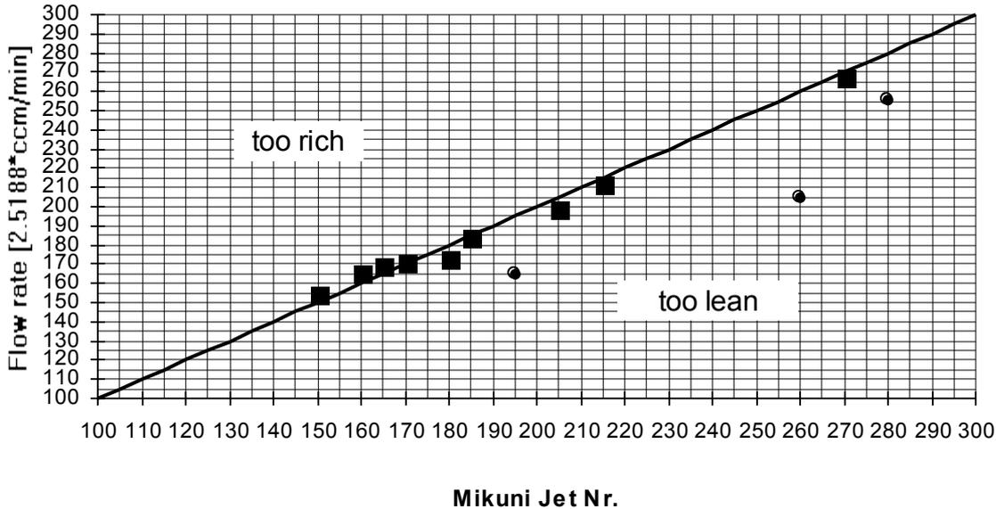
Figure 22: Reference straight for the corrected flow rate
