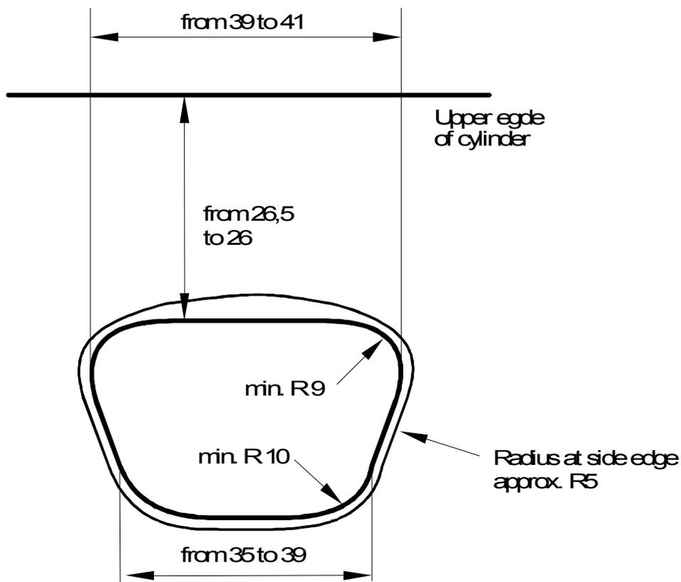
Figure 67: Exhaust port seen from the cylinder
