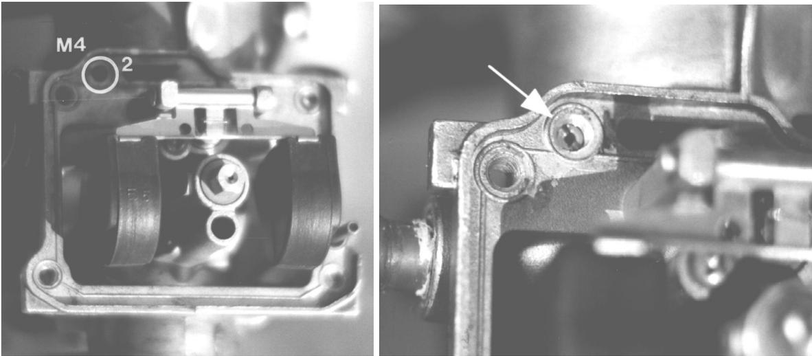
Figure 19: End of passage 2 (left: stock, right: modified)
