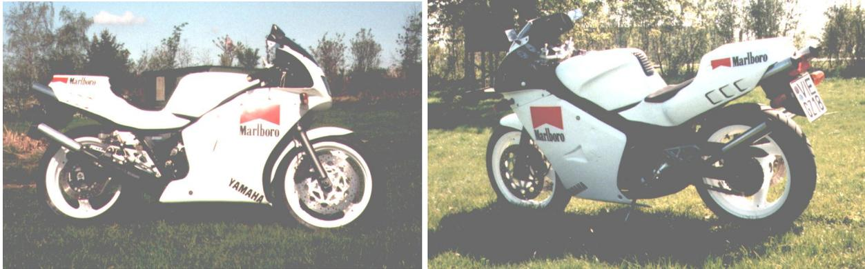
Figure 106: Klöpper RD500 (FZR conversion, RGV Bodywork, Jolly pipes)
