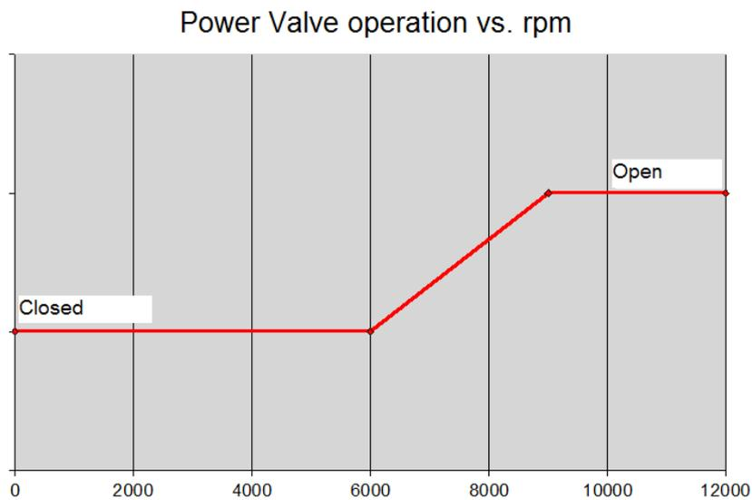
Figure 90: Power-Valve operation vs. engine-rpm (RZ350)
