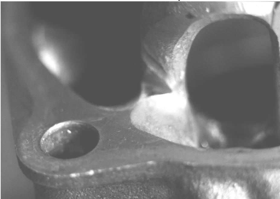
Figure 58: Region between boost port and transfer port
