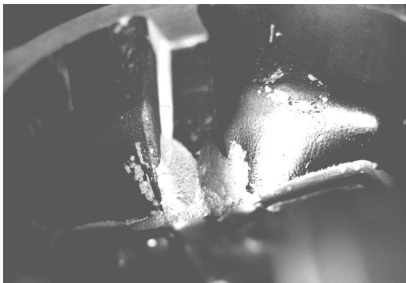
Figure 50: Continuation of intake port bridge in the crankcase
