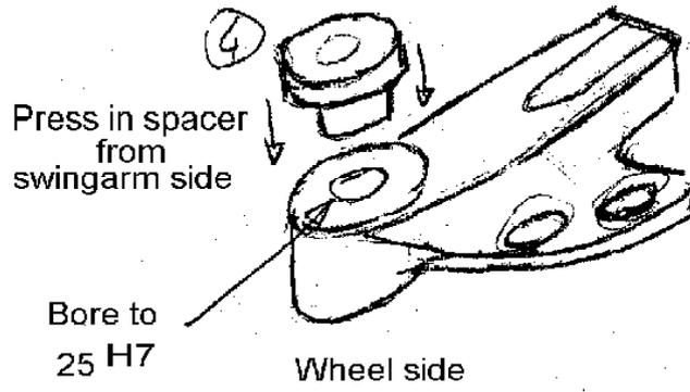
Figure 120: Press in brake carrier spacer from swingarm side
