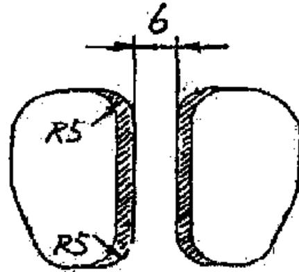
Figure 47: Modified intake port shape (YAMAHA race specs)
