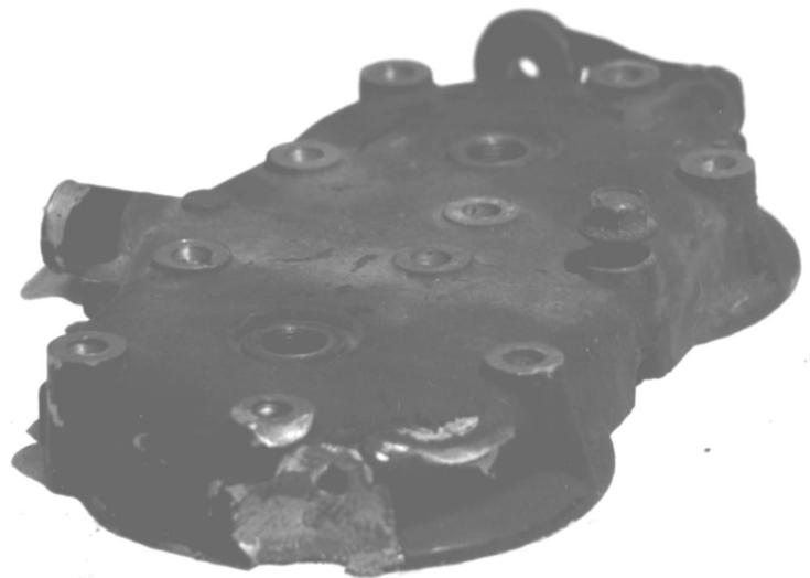
Figure 7: Damaged lower cylinder head
