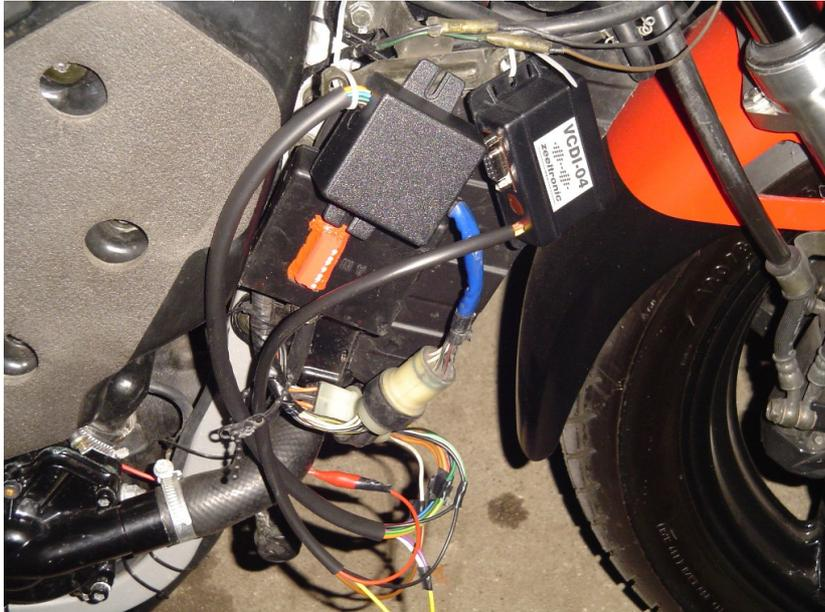
Figure 86: CDI (left), VCDI (middle) (prototypes from [www.zeeltronic.com](http://www.zeeltronic.com))
