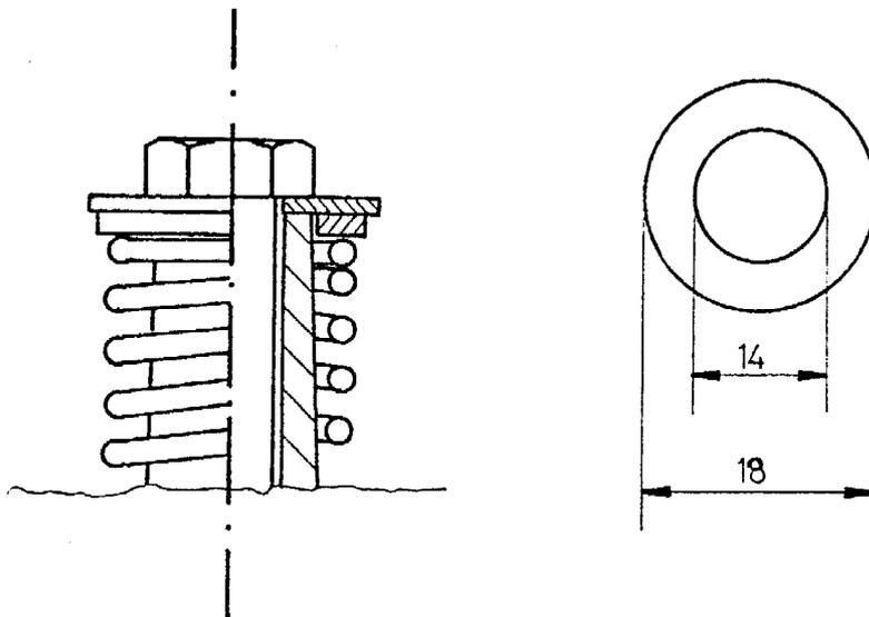
Figure 80: Clutch spring with washer
