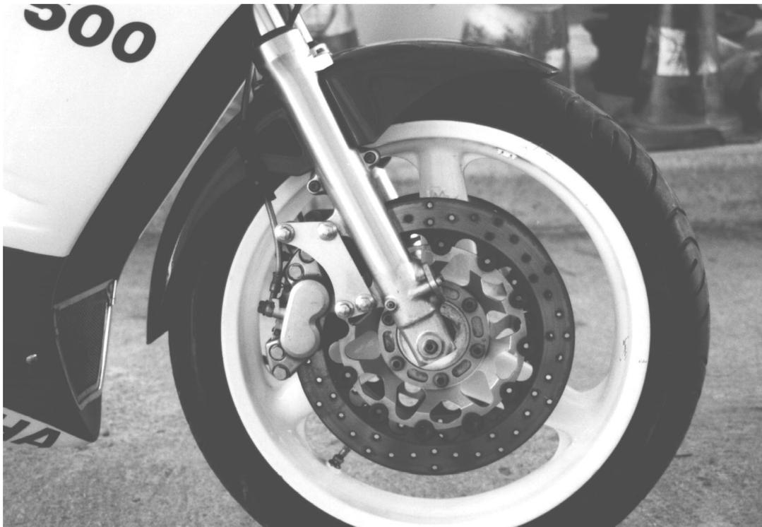
Figure 105: FZ wheel and brakes in RD500 fork (anti dive closed)
