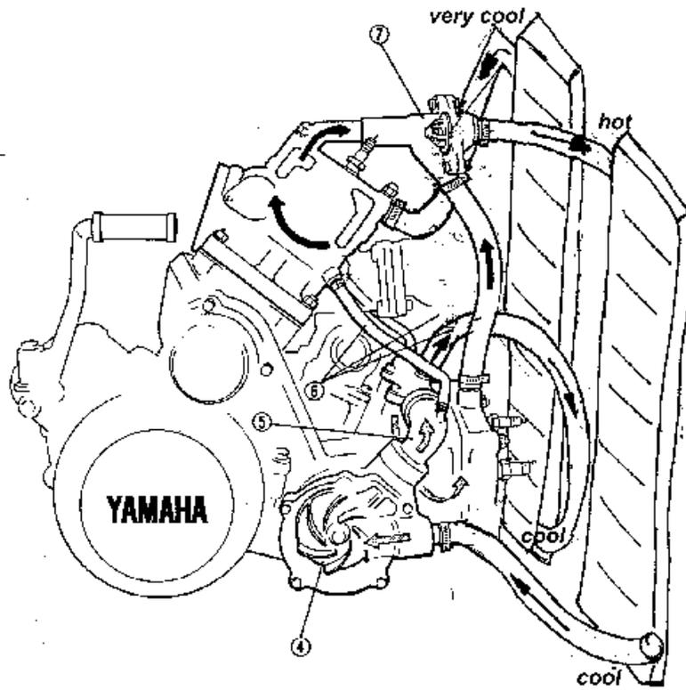
Figure 78: Concept with two radiators
