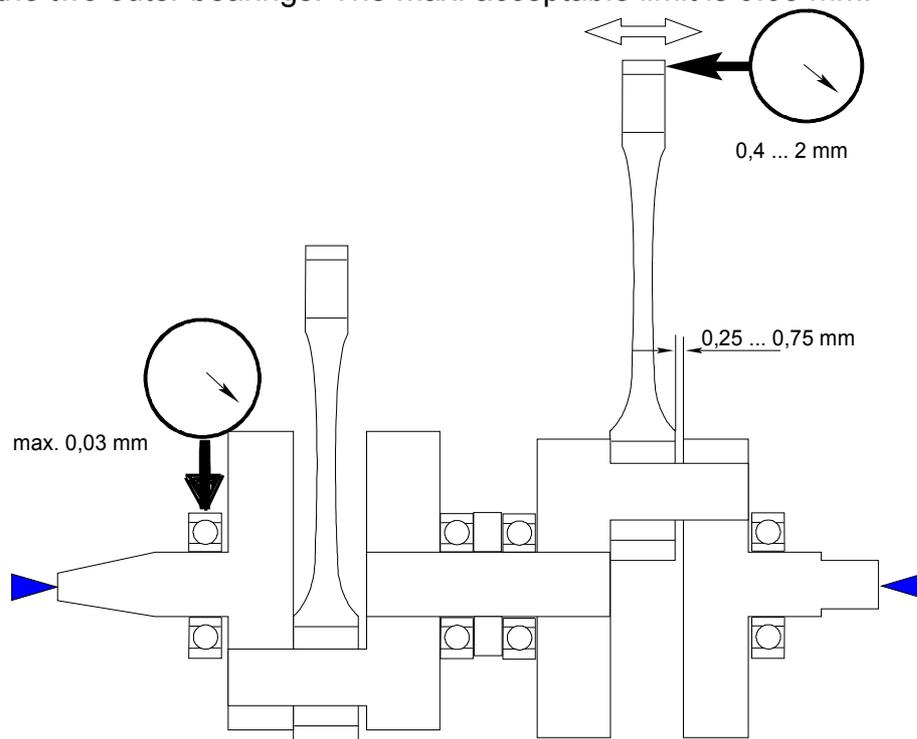
Figure 4: Crank tolerances
