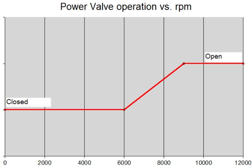
Figure 90: Power-Valve operation vs. engine-rpm (RZ350)
