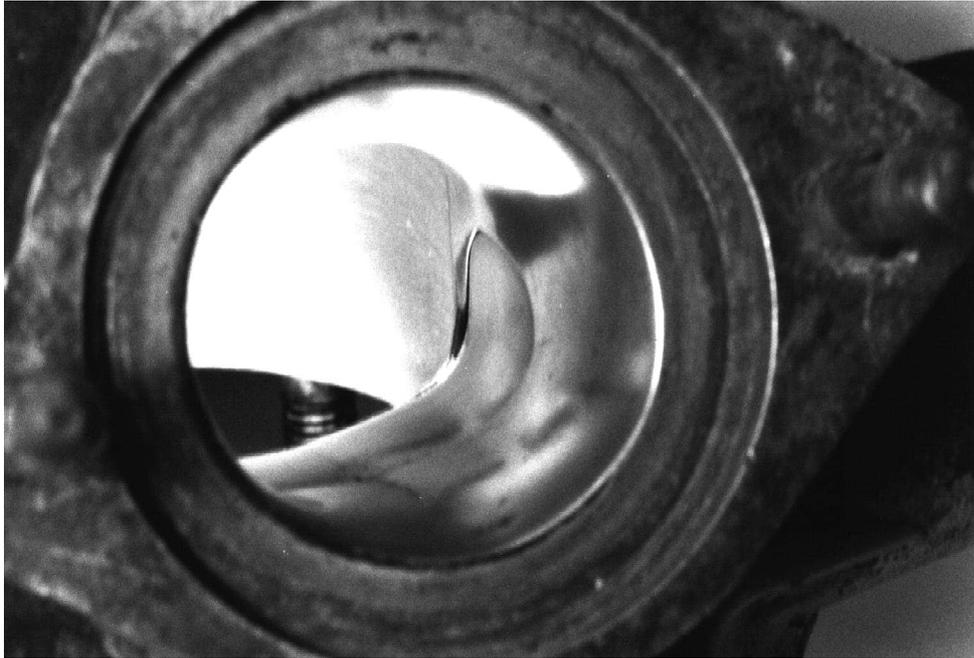
Figure 70: Exhaust port machined and polished (RD350)
