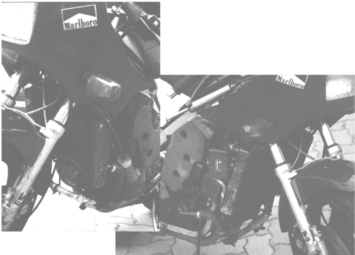
Figure 79: GXSR750W radiator fit to RD500
