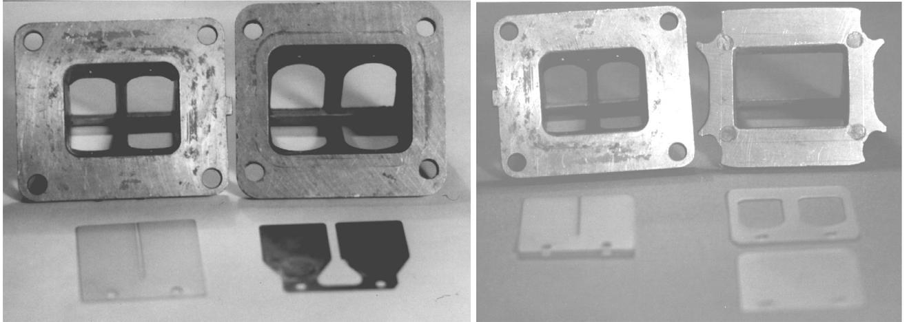
Figure 46: Left: RZ350 cages, Right: CR80 cages with bridge removed
