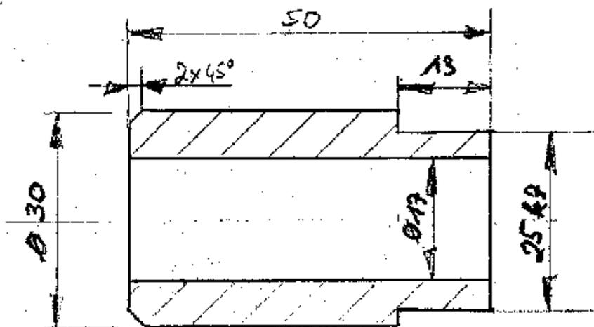
Figure 119: Bearing spacer in the sprocket carrier
