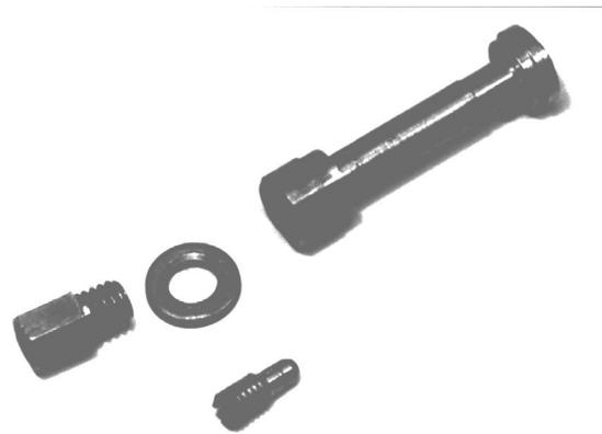
Figure 11: Nozzle, main jet, idle jet
