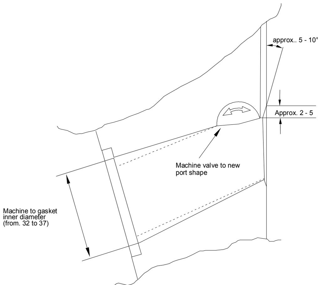
Figure 68: Cross section along flow way
