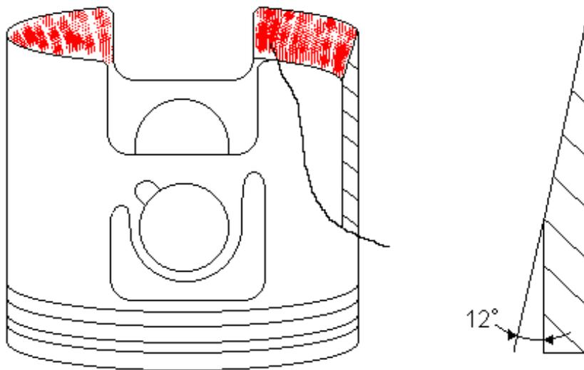
Figure 54: Piston skirt cross section after machining
